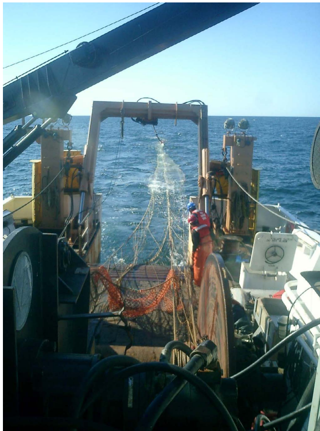
Figure 2. Pelagic trawl, provided by the National Marine Fisheries Service, streaming out behind the ship before being lowered down to depth.
