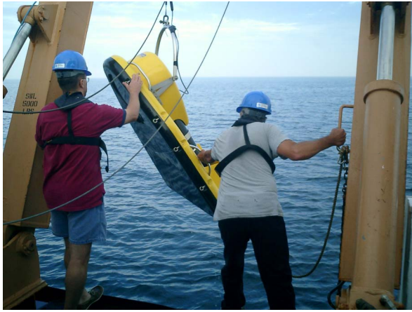
Figure 1. Edgetech towbody being deployed for use during the September 2005 cruise on the FR/V Delaware II. The system was towed near the surface, deep in the water over fish schools, and deep in the water through fish schools.
