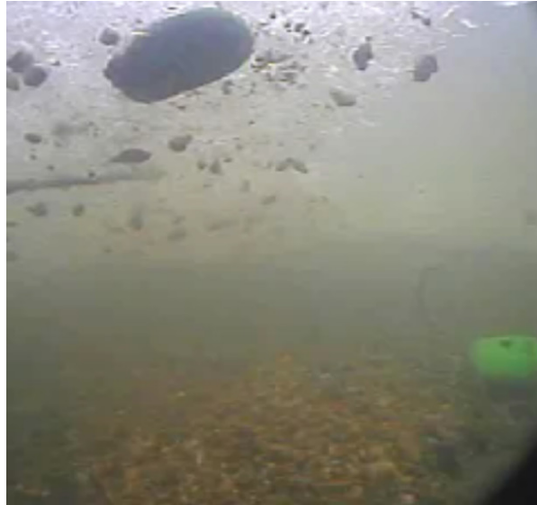
Figure 1. Still image from an underwater video showing two of the tracer cobbles used to monitor ice rafting in the Laramie River, WY. One bright-green tracer (mass: 263 g) is visible on the bed in the lower right portion of the image. The other tracer (830 g, at the top center of the image), along with assorted gravel, is suspended 30 cm above the river bed in a recently released anchor ice mass. The video clip can be viewed at http://faculty.gg.uwyo.edu/kempema/vidtour.html
