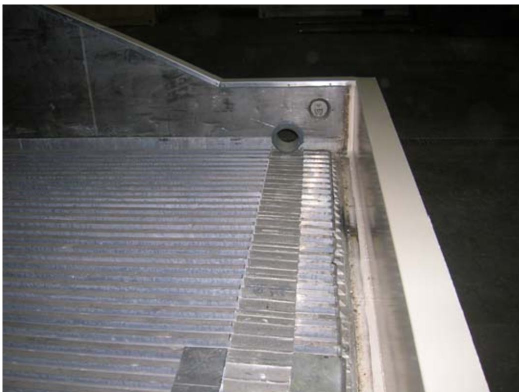
Figure 12. Interior view of the completed field lysimeter demonstrating the leachate collection system.
