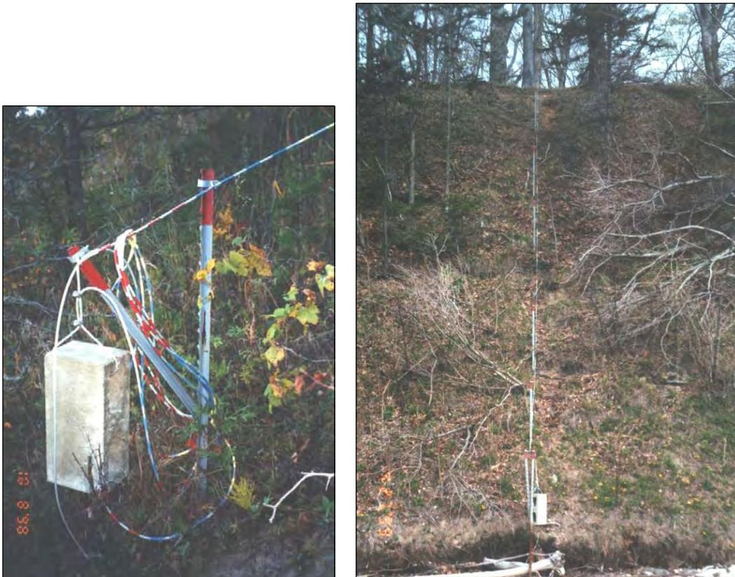
Figure 18. Last pole, left, of the calibrated pole-cable system and concrete anchor, and, right, calibrated cable system shortly after installation at 116<sup>th</sup> Avenue.
