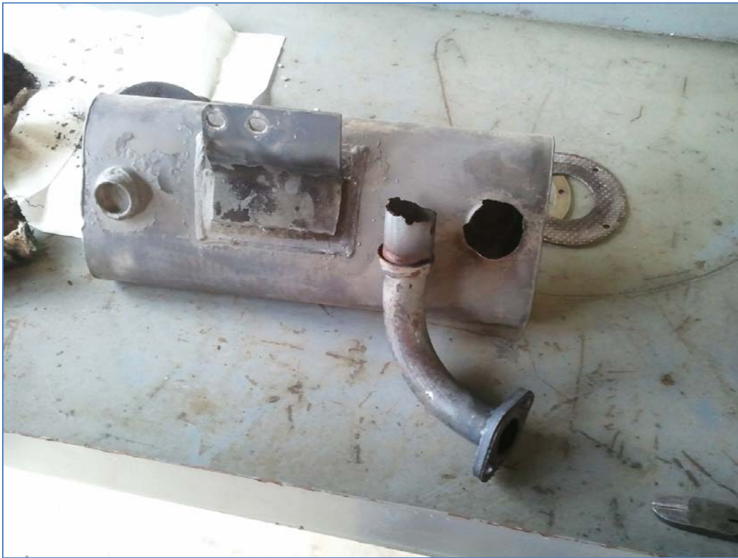
Figure 3. Muffler and Header Pipe Showing Broken Welds as a Result of the Muffler Bolt Failure
