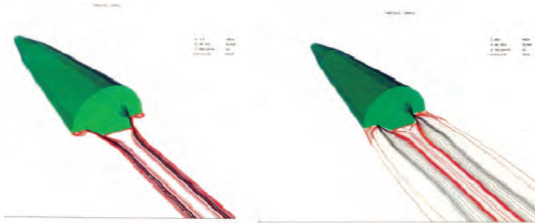
Figure 4. Plug nozzle plume studies, 0.0 degree angle-of-attack, free stream Mach number 0.32
