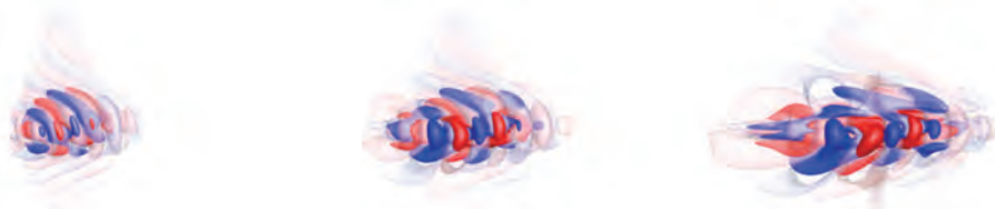
Figure 9. Downstream evolution of wave packet resulting from high-amplitude of forcing oblique mode with \beta=10 . Shown are iso-surfaces of the streamwise disturbance velocity |u'|=10^{-2} and 10^{-3} at t=5.76s (left), 7.68s (center), and 9.6s (right).
