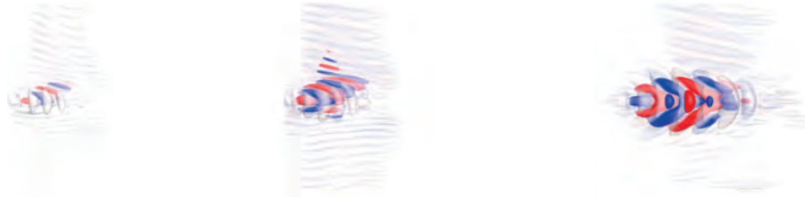
Figure 10. Downstream evolution of wave packet resulting from high-amplitude forcing of oblique mode with \beta=20 . Shown are iso-surfaces of the streamwise disturbance velocity |u'|=2 \cdot 10^{-3} and 2 \cdot 10^{-4} at t=5.76\text{s} (left), 7.68\text{s} (center), and 9.6\text{s} (right).
