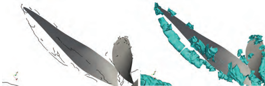
Figure 3. Automatically generated: (a) vortex corelines, (b) surfaces
