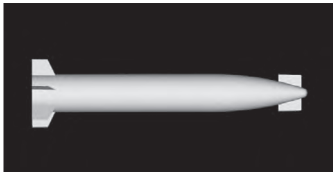
Figure 8. Canard-controlled finned projectile geometry
