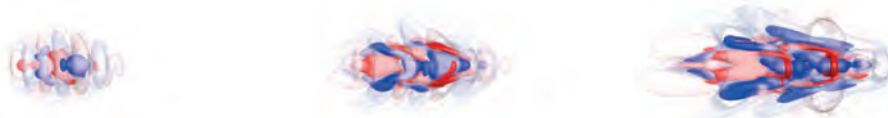
Figure 8. Downstream evolution of wave packet resulting from high-amplitude forcing of oblique mode with \beta=2 . Shown are iso-surfaces of the streamwise disturbance velocity |u'|=5*10^{-2} and 5*10^{-3} at t=5.76s (left), 7.68s (center), and 9.6s (right).
