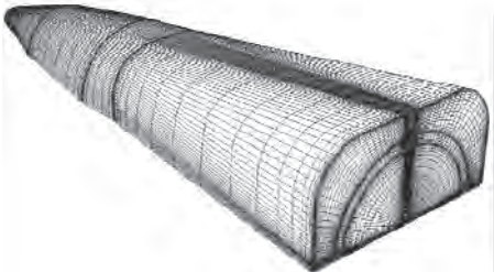
Figure 1. Traditional conical body with embedded bell nozzle rocket
