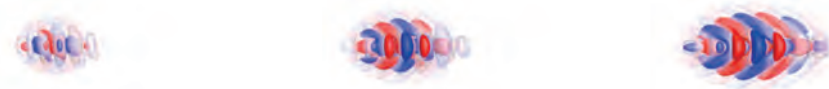
Figure 7. Downstream evolution of wave packet resulting from low-amplitude forcing of oblique modes with \beta=0-40 . Shown are iso-surfaces of the streamwise disturbance velocity |u'|=5*10^{-7} and 10^{-7} at t=5.76s (left), 7.68s (center), and 9.6s (right).
