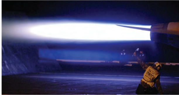
Figure 1. Aircraft carrier flight deck crew at takeoff (F/A-18E/F Superhornet). Full-cranial hearing protection is worn by all visible personnel. Jet blast deflector is visible at left.
