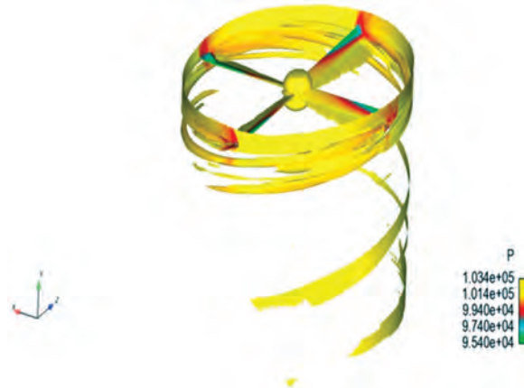
Figure 8. Iso-surface of vorticity colored by pressure
