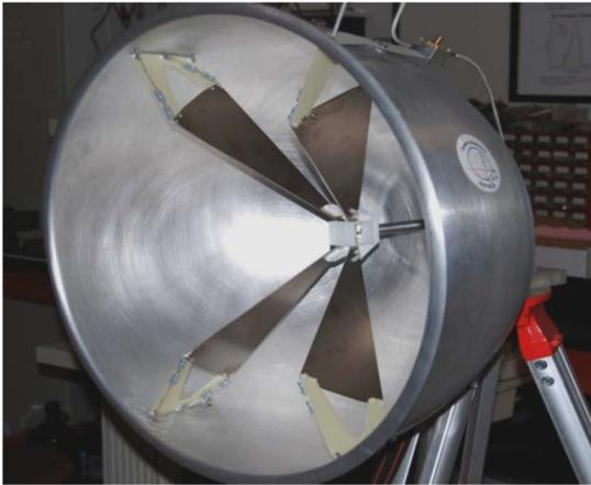
Fig. 1. Antenna structure. (a) Side view. A differential signal is fed to the transmission line at the first focal point ( $-z_0$ ). (b) Front view.  $\phi_0$  is the angle between the feed-arm and y-axis. (c) The actual antenna.
