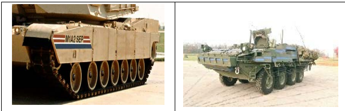
Figure 32. Comparison of Tracked (Left) (From Cooke 2008) and Wheeled (Right) (From Cooke 2009) Propulsion Systems
