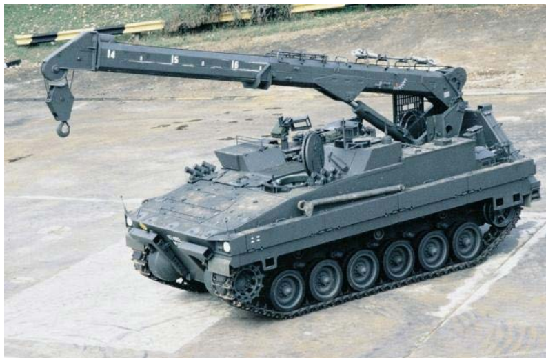
Figure 63. Recovery Variant of the Bionix IFV (From IHS Jane's 2011)
