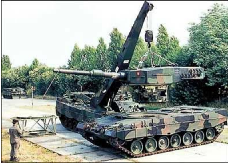
Figure 65. Removal of a Leopard 2 MBT Turret (From The Armor Site, n.d.)
