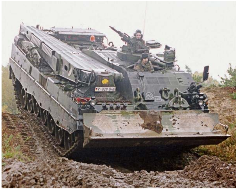
Figure 62. The Buffel Armored Recovery Vehicle (ARV), a Variant of the Leopard 2 MBT (From IHS Jane's 2012)
