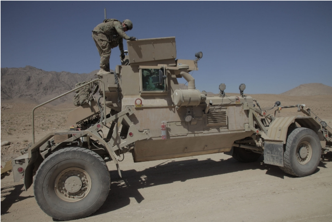
Figure 17. A Husky Mk III. Notice the Sloped Bottom Hull, an Example of the V-Shaped Hull (From Critical Solutions International, 2012)
