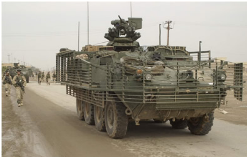
Figure 16. A Stryker IFV Mounted with Slat Armor (From Defense Update Jan 2006)
