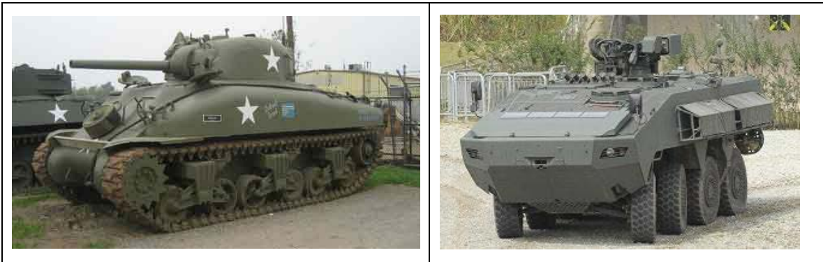
Figure 33. Illustration of Traditional Turret Mounted Gun (Left) (From Zimbio, n.d.) vs Remote Controlled Weapon Station (Right) (From Ministry of Defence, Singapore 2009)
