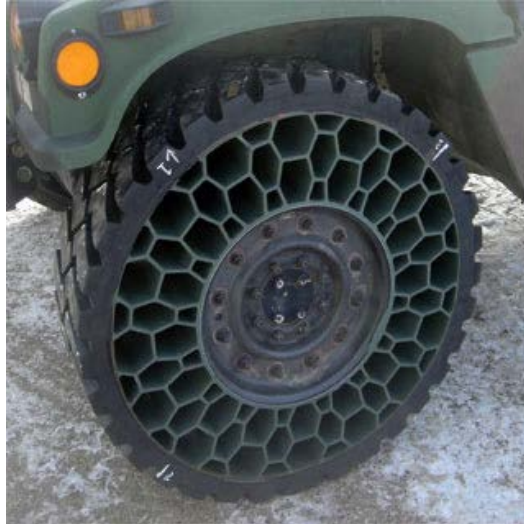
Figure 59. An Example of Airless Tyre Installed on a Humvee (From Greenemeier 2008)
