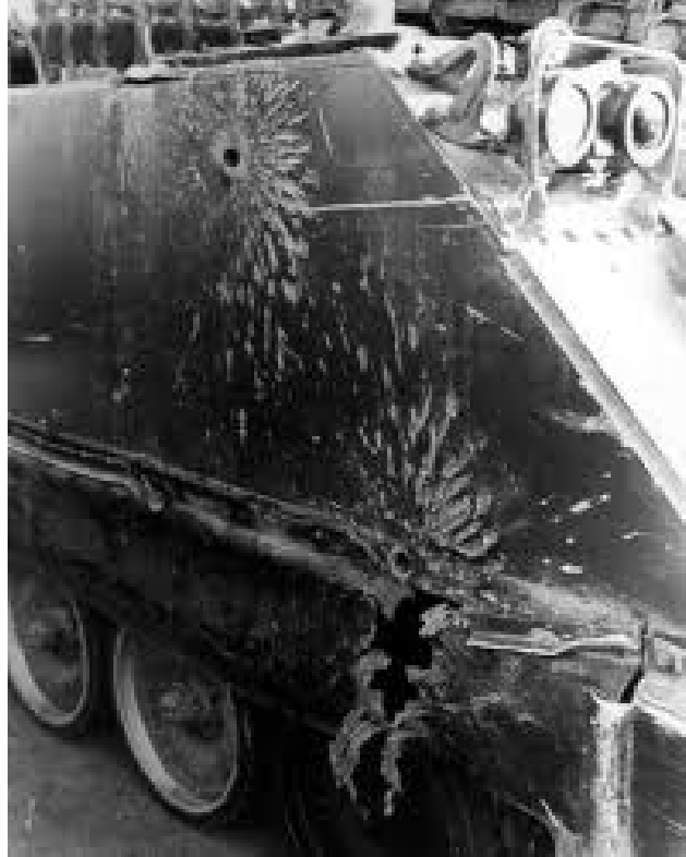
Figure 12. An M113 with Hits from a Viet Cong 57mm Recoilless Rifle (From Starr 1980, 46)
