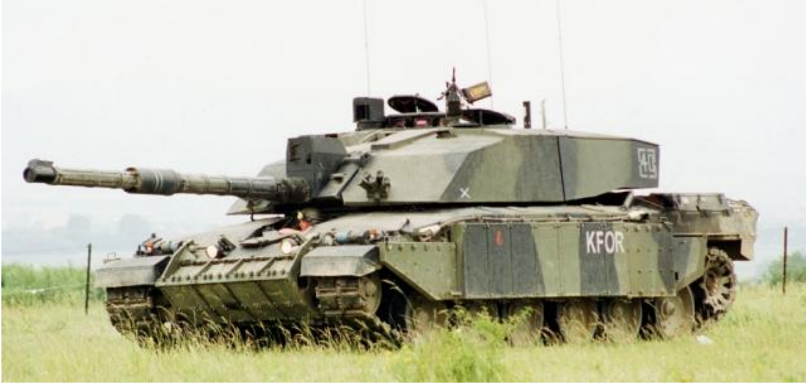
Figure 42. A Challenger 2 MBT (Note the Thicker Side Skirt) (From IHS Jane's 2012)
