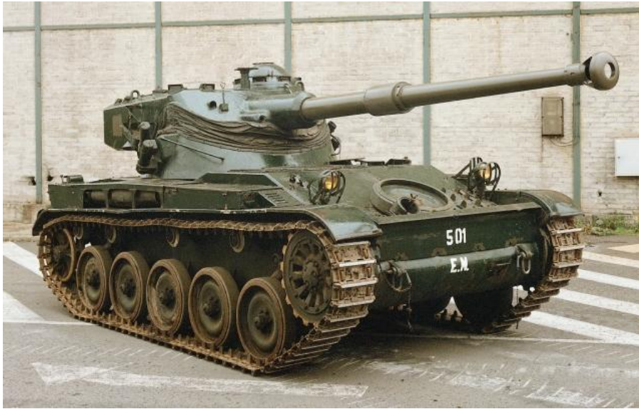
Figure 39. An AMX-13 Light Tank (Note the Sloped Front Side of the Turret) (From IHS Jane's 2012)
