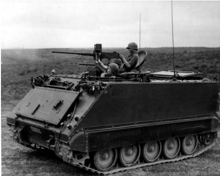
Figure 10. A Typical M113 Operated by the South Vietnamese Army (Shown without Gun Shield) (From Starr 1980, 23)
