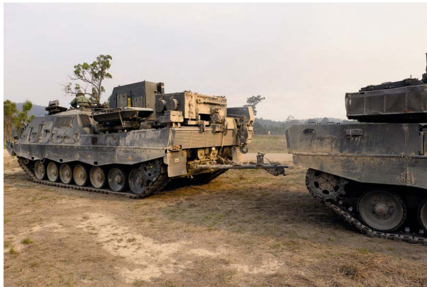
Figure 64. A Buffel ARV Hooking up an Incapacitated Leopard 2A4 MBT Using the Combat Recovery Device (From Ministry of Defence, Singapore 2012)
