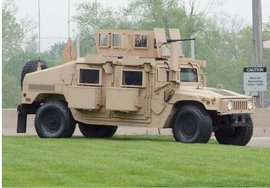
Figure 5. A M1151 Mounted with the Frag Kit 6, an Example of an Up-Armored Light Vehicle (From IHS Janes's 2012)
