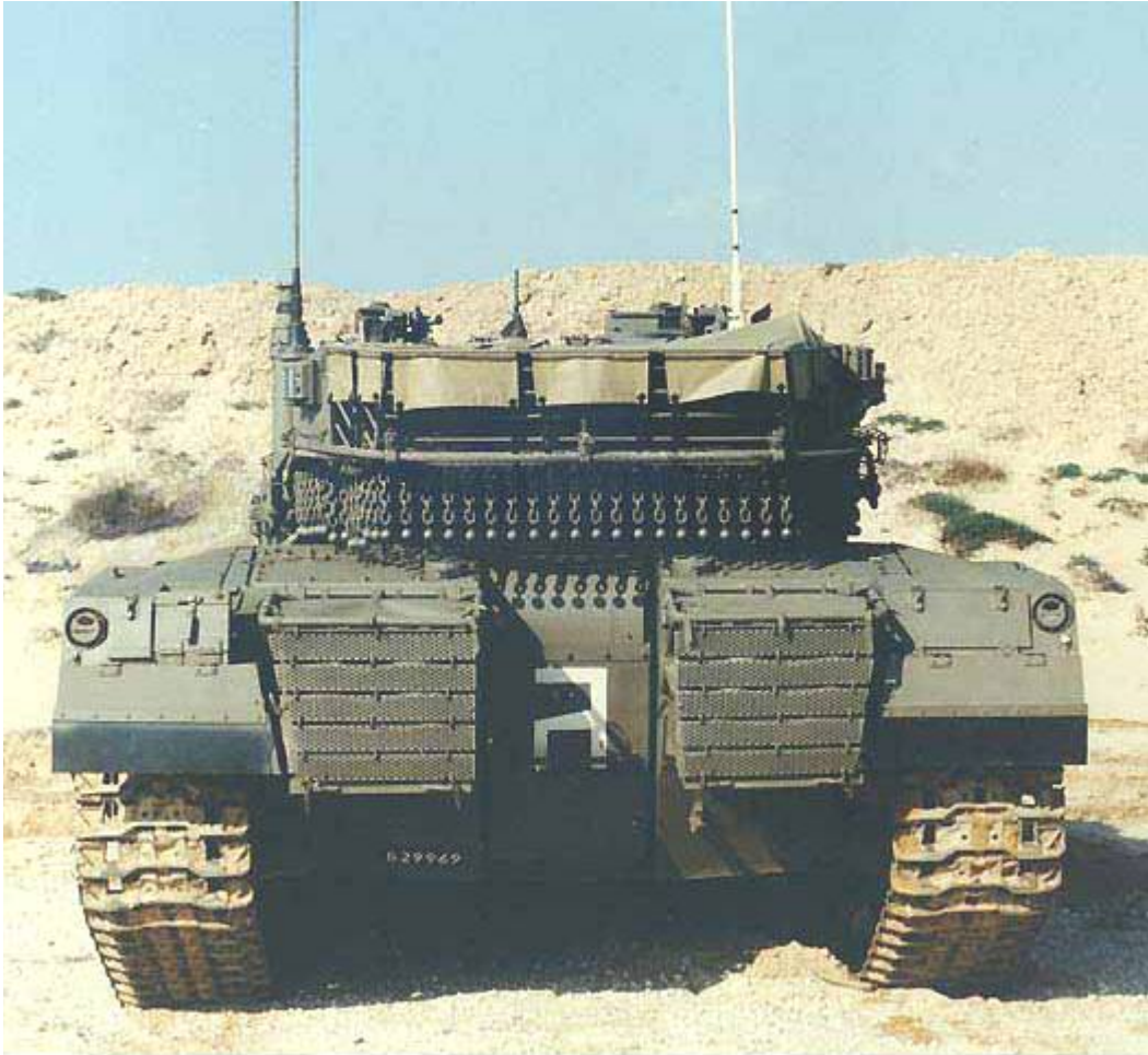
Figure 53. A Rear View of the Merkava Mk III. Notice the Curtain of Chain Links Hanging from the Turret. (From Army-technology.com 2011)
