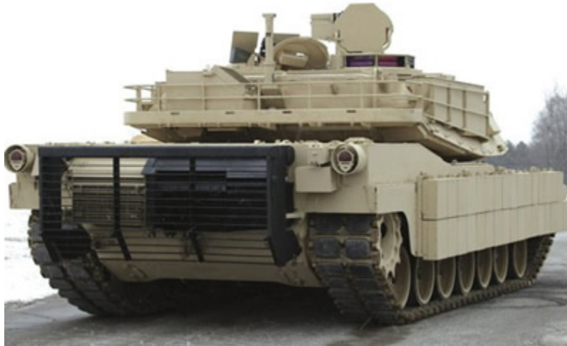
Figure 18. An M1 Abrams MBT Mounted with a TUSK (From Defense Update Dec 2006)
