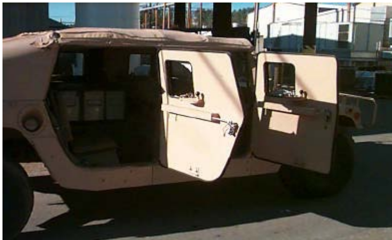
Figure 15. Armor Plate Doors Mounted on the Humvee as Part of the ASK (From U.S. Army (TACOM) 2004, 5)
