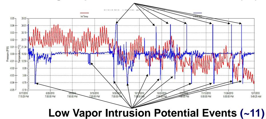
Blue line – Pressure differential (Subsurface to Indoor) Red line - Subsurface temperature
