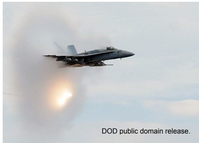
FIGURE 97. Flare Dispensed in Transonic Flight. (An F/A-18C drops flares during an air power demonstration aboard the USS Dwight D. Eisenhower [CVN 69], 27 July 2010. Decoy countermeasures will continue to play a major role in aircraft defense for at least the next decade.)
