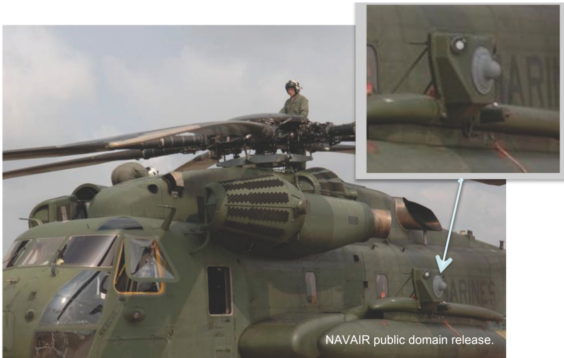
FIGURE 9. LAIRCM on CH-53E. (Marines in theater conduct maintenance on a CH-53E equipped with LAIRCM.)
