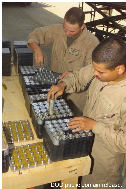
FIGURE 73. Ordnancemen Inspect and Replace Expended Flares Out of Chaff and Flare Buckets of KC-130, 10 March 2002, in Support of Operation Enduring Freedom.
