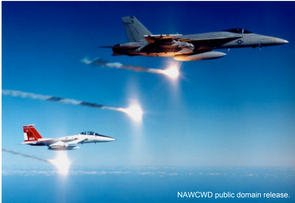
FIGURE 70. Conventional Pyrotechnic Flares Dispensed From F/A-18E.
