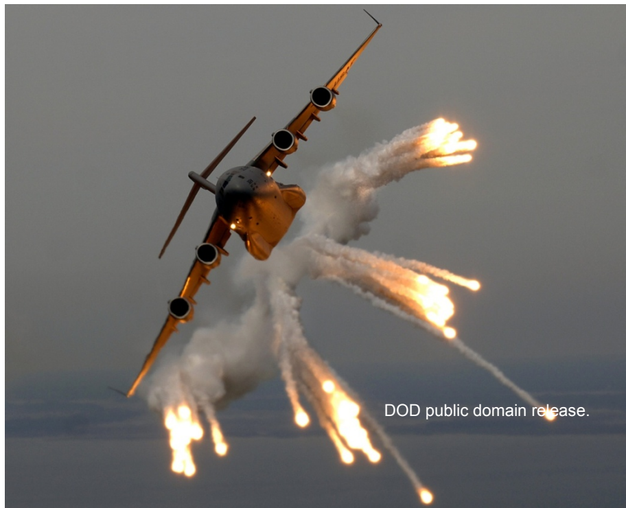
FIGURE 5. Flare Salvo From C-17. (A C-17 Globemaster III aircraft releases flares over the Atlantic Ocean during a local exercise over Charleston, South Carolina, 6 May 2006.)
