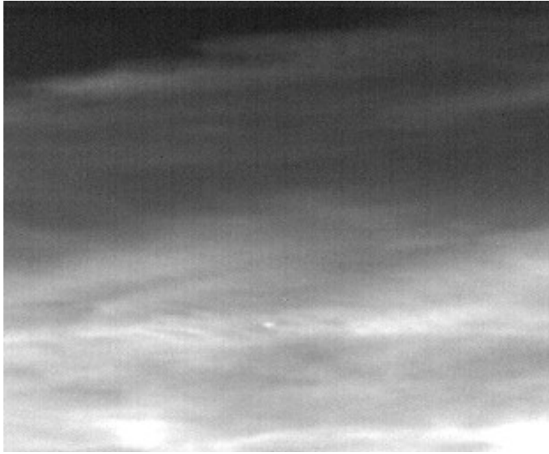
FIGURE 38. Aircraft IR Image at Missile Acquisition Range. (Ground-to-air IR image of an aircraft nose-on against broken cloud background at a range of 7.6 nautical miles taken with a commercial IR camera.)
