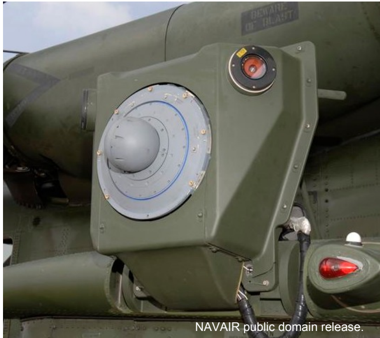
FIGURE 89. Close-up of LAIRCM System Installed on CH-53E.
