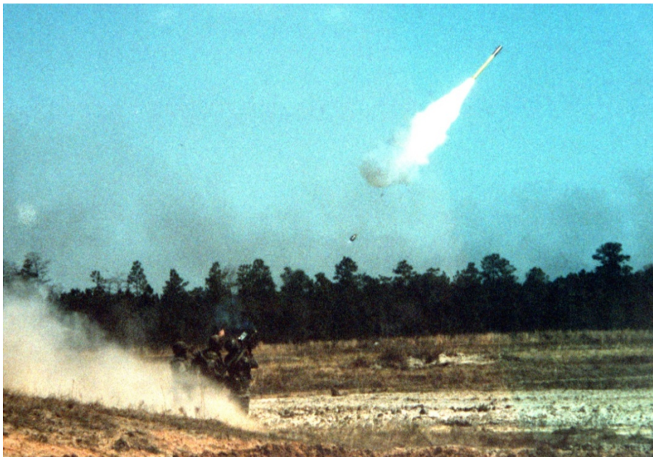
FIGURE 94. U.S. Army Stinger Launch During Live Fire Exercise. (The open flame of rocket motors emit radiation across the spectrum from UV through MWIR.)
