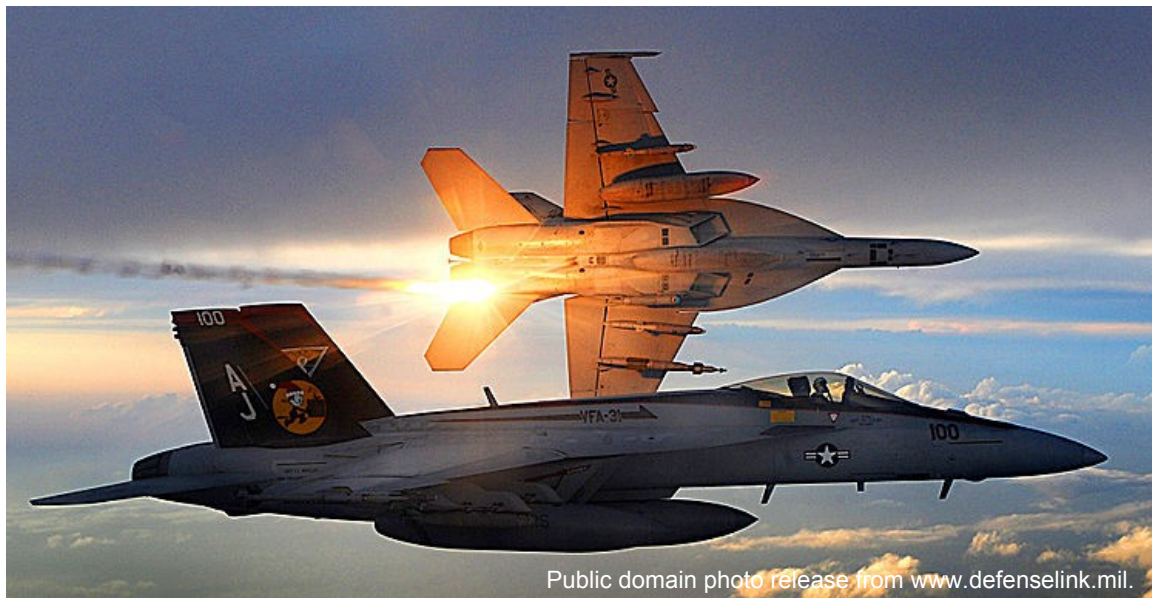
FIGURE 69. Conventional Pyrotechnic Flare Dispensed by Navy F/A-18E.
