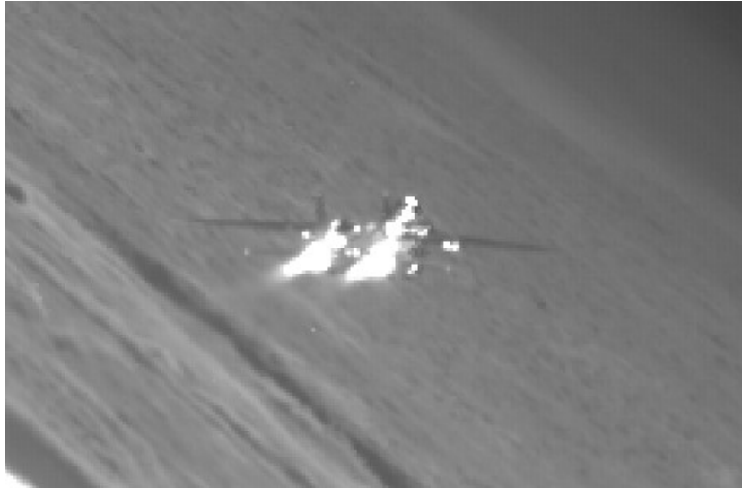
FIGURE 37. Aircraft IR Signature Complexity. (MWIR image of F-14A showing engine dominance at tail, solar reflections from the top of the fuselage, and sky reflection from the top of the wing surfaces.)
