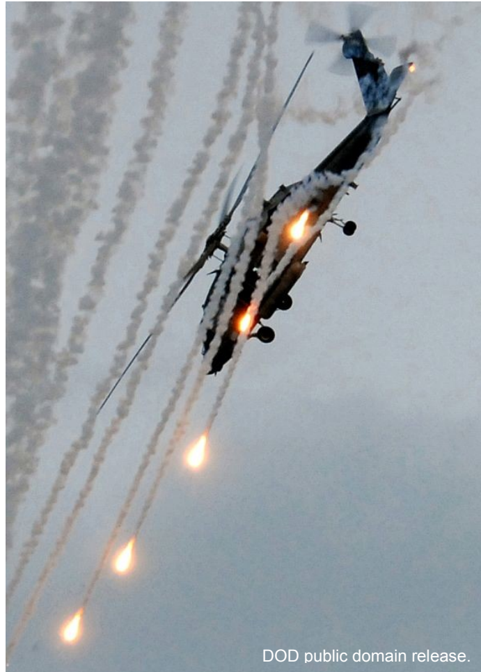
FIGURE 102. Flare Salvo From HH-60H Sea Hawk. (An HH-60H displays the ability to launch flares and quickly maneuver during an air power demonstration from the USS Ronald Reagan [CVN 76].)
