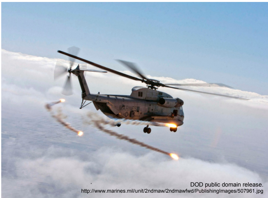
FIGURE 68. Marine Corps CH-53D Dispenses Pyrotechnic Flares.
