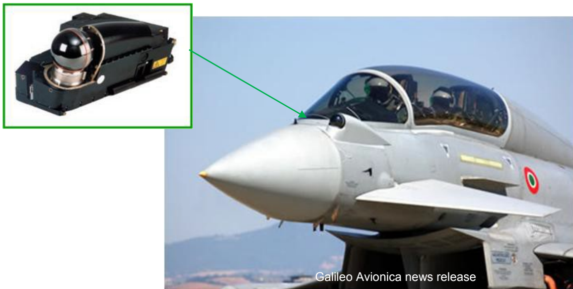
FIGURE 101. PIRATE IRST System on Italian Eurofighter. (The European PIRATE is one of a new generation of fighter IRST systems. Combined with long-range IR missiles, these devices will allow passive BVR attack.)
