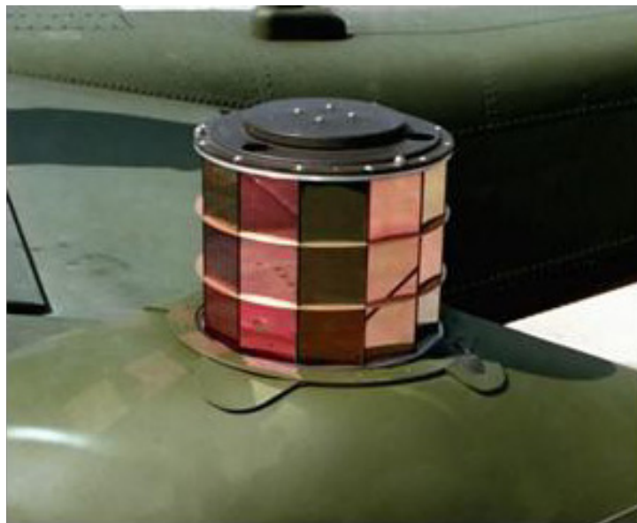
FIGURE 80. ALQ-144 on OV-10D.
