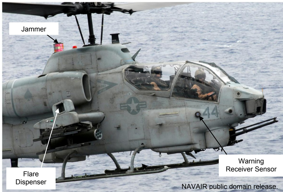
FIGURE 92. IRCM Suite on AH-1W Super Cobra. (IRCM installations on an AH-1W, 17 October 2008, over flight deck of USS Peleliu .)
