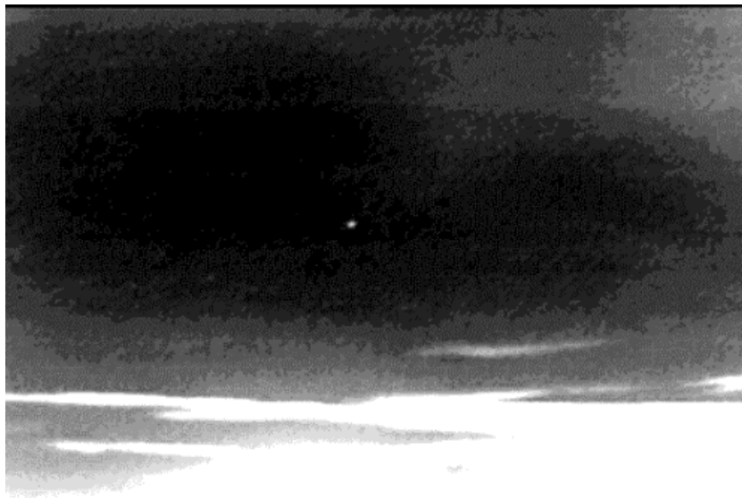
FIGURE 2. Image of Aircraft Nose-on at 23-Nautical-Mile Range Taken With Commercial IR Camera.
