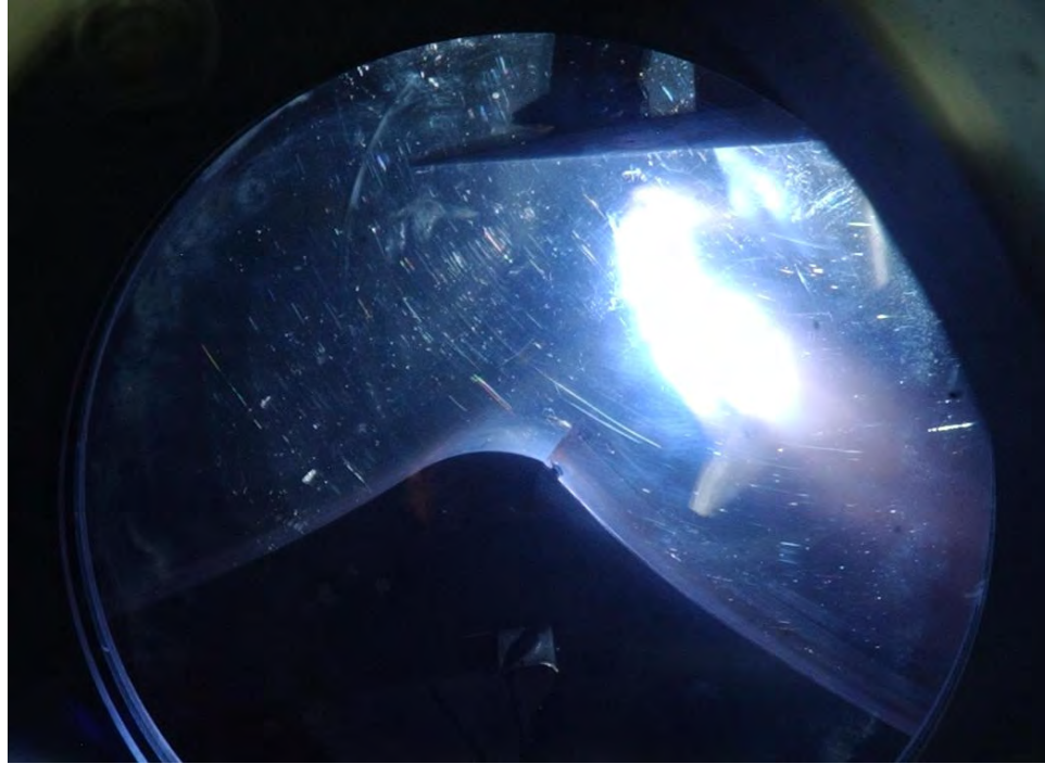
Figure 5.16: Run#17 - Long exposure color photograph of laser-induced breakdown geometry at Mach 5.96; 2D model at -7.5^\circ ; Shroud at -4^\circ inclination.
