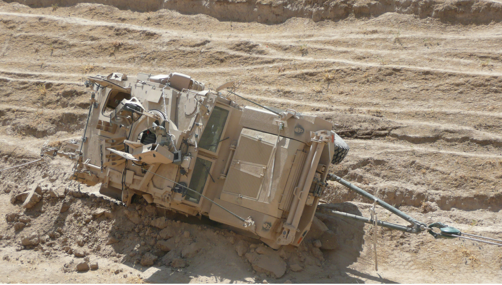
After hours of attempting more delicate procedures to remove the vehicle, the recovery team resorts to pulling the RG-31 from the ditch using a heavy expanded-mobility tactical truck's winch and a 60-ton snatch block.
