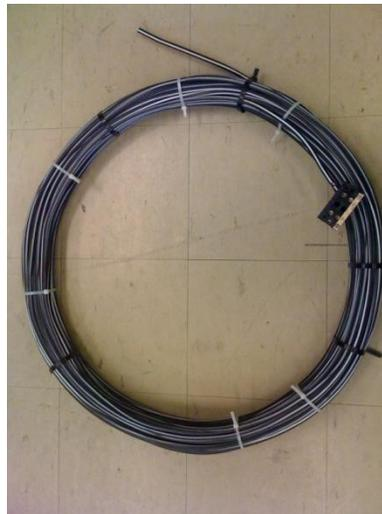
However this will result in a very bulky Helmholtz coils. The above design has less than 50 turns. The Helmholtz coil will have turns on the order of  $10^2$ . Thus such heavy insulation may not be feasible since we want the coil to fit around the air bearing but within the frame. Also enamel coated wire may or may not do the job.
