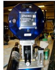
Another demo called “StopAndStare” focused on the attitude control instead of the position control. This demonstration showed the ability to control the attitude as well as the gain. In the demo, SPHERES was controlled to have only 10° of overshoot in its attitude. These two demos were good experience for when SPHERES will be used to test components on the air bearing.
