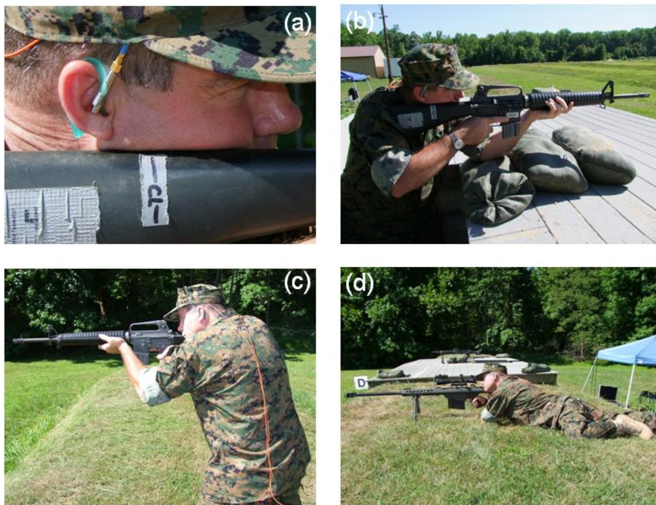
Fig. 16 — Photos showing (a) ear clip attachment to ear. Measurements were made with a human wearing the ear clips from (b) foxhole, (c) standing and (d) prone positions.
