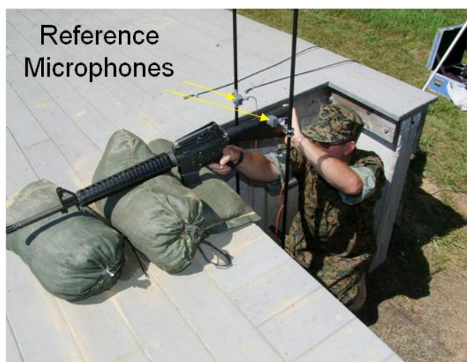
Fig. 11 — Acoustic reference configuration in foxhole. The two microphone positions represent head center references for the left and right handed shooter.
