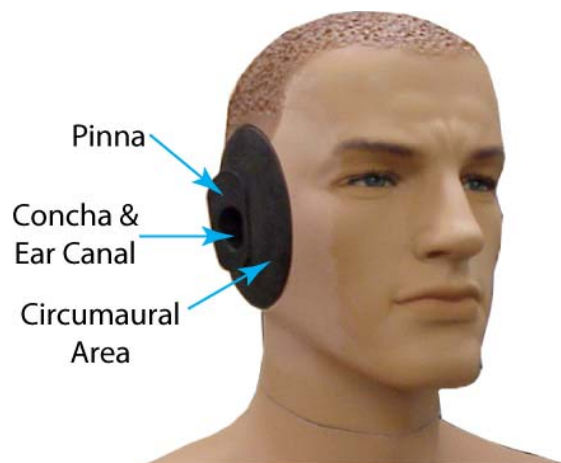
Fig. 1 — Surrogate head with both ears modeled including circumaural area, pinna, concha, ear canal, and high dynamic range pressure sensors (not shown) at the end of each ear canal chamber.
