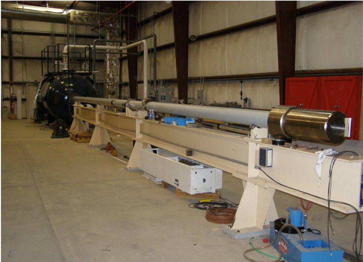
Figure 2.1: The HP3 60mm gun
