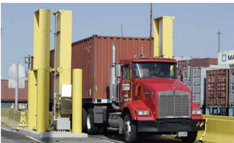
A truck passes through a radiation portal monitor during a security screening at the Port of Tacoma in Washington State.
