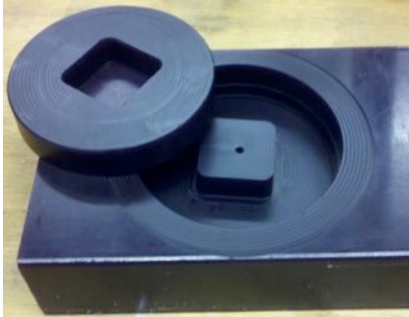
Figure 63: Wax mold for hysol molding process.
