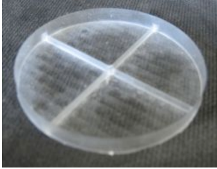
Figure 61: Example acrylic vehicle structure with stiffening ribs.
