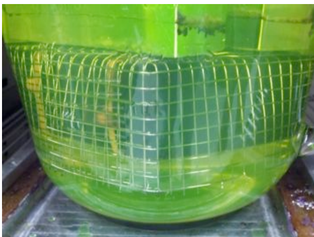
Figure 65: Glycol bath used to remove mold material from hysol vehicle structure.
