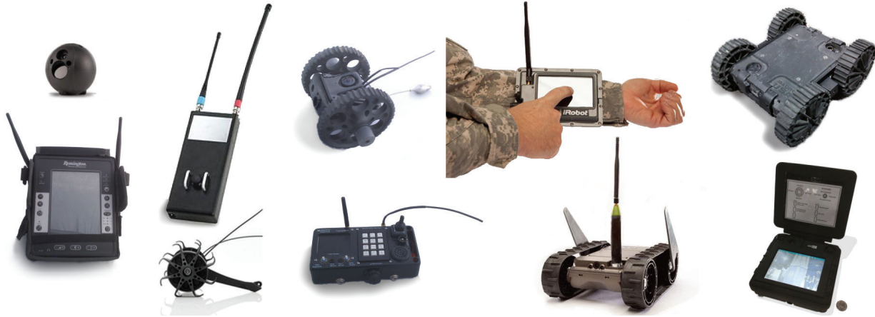
Figure 2. The robots used in the tests and their OCUs, left to right: ODF Optronics EyeBall , ReconRobotics Recon Scout XT , Omnitech Robotics Toughbot , iRobot FirstLook , and MacroUSA Armadillo .
