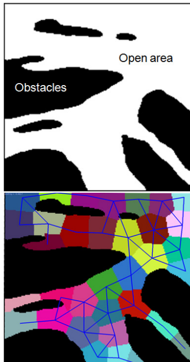
Figure 8: KML automatically subdivides the total area into smaller areas called “countries”, each with a “capital”. From the capital the robot can see the entire country, given the known obstacles.
