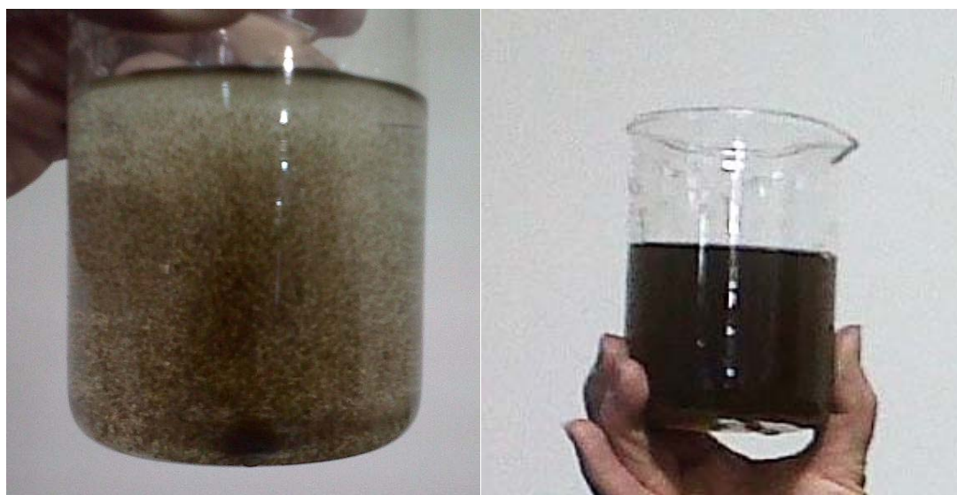
Figure 15. Fluid recovered from water-only backwash at 12 psi (left), and water recovered through combination of water backwash with bore-side air scour (right)
