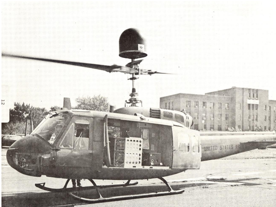
Army Helicopter with SHF SATCOM Terminal
