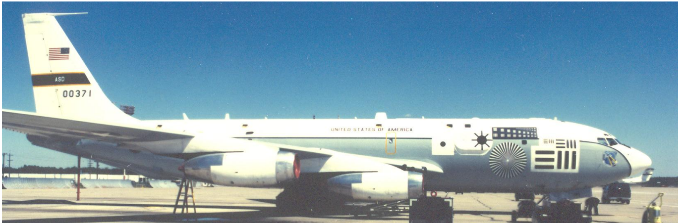
Figure 5b 4950 th Test Aircraft C-135-371 With Optical Window
