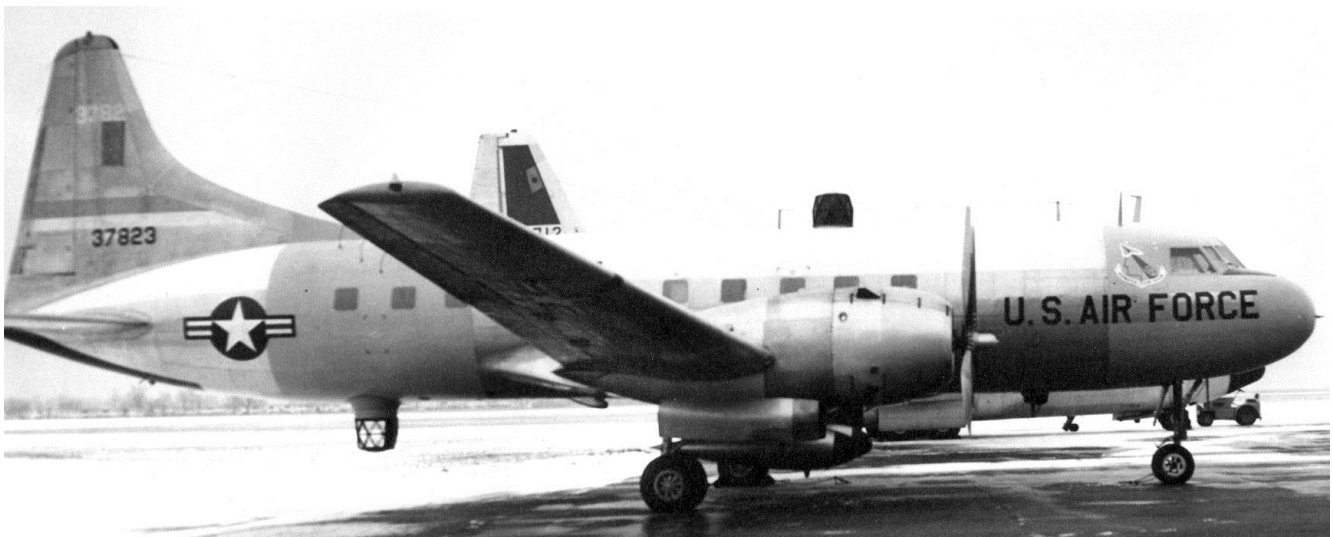
C-131 Test Aircraft with Top and Bottom IR Radomes
