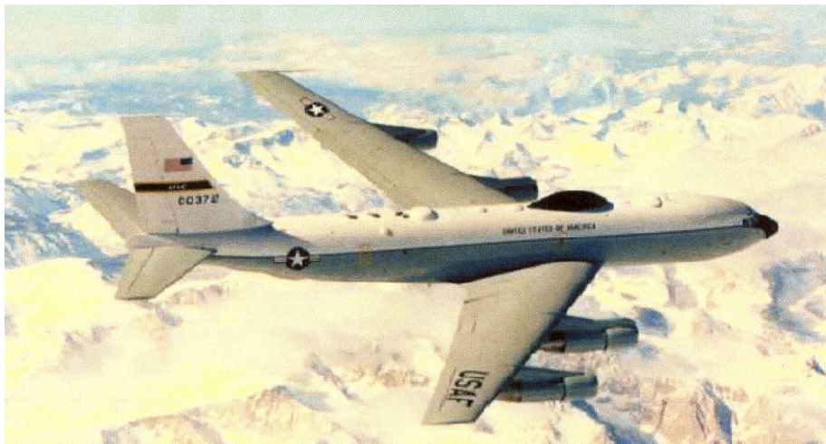
Figure 2 AFRL SATCOM Test Aircraft with Luneberg Lens Antenna under White Radome
