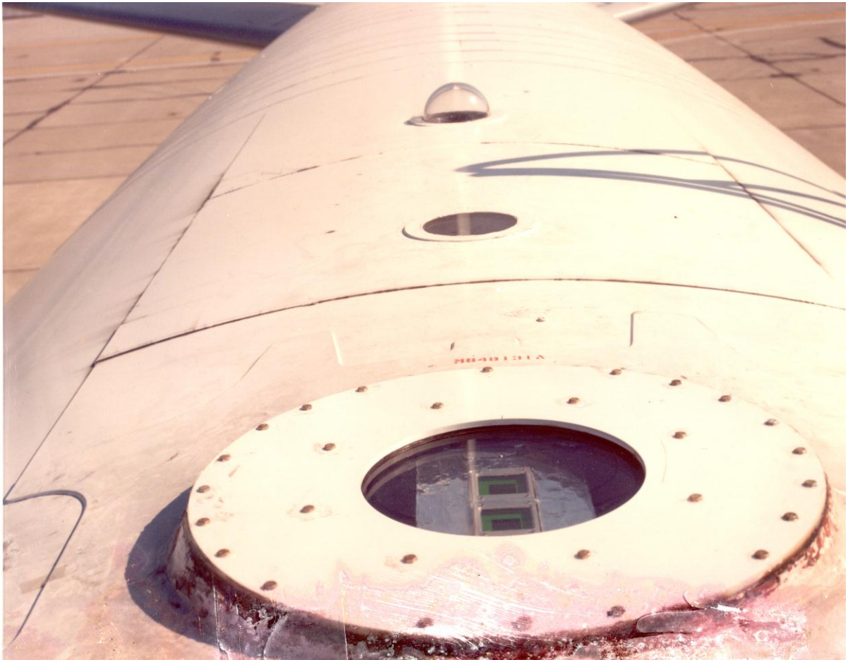
Figure 6b Receiver Aircraft (C-135-3131) with Top-mount Receiver
