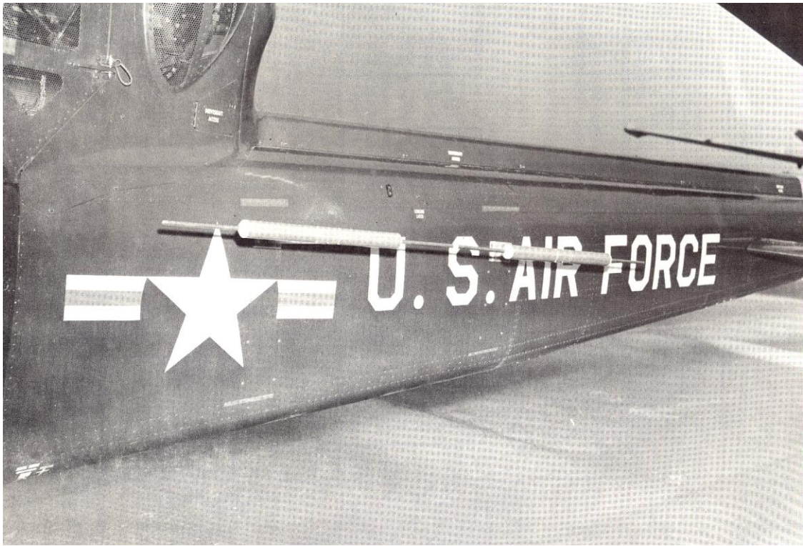
VHF Horizontally Polarized Antenna on Helicopter
