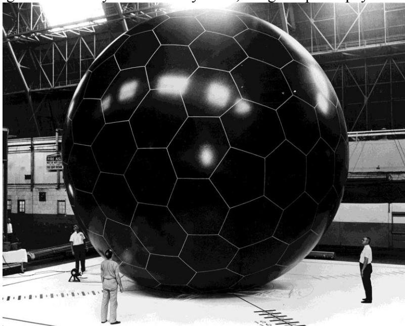
Figure 4 Thirty-foot Diameter Grid Sphere Similar to One Launched into Orbit
