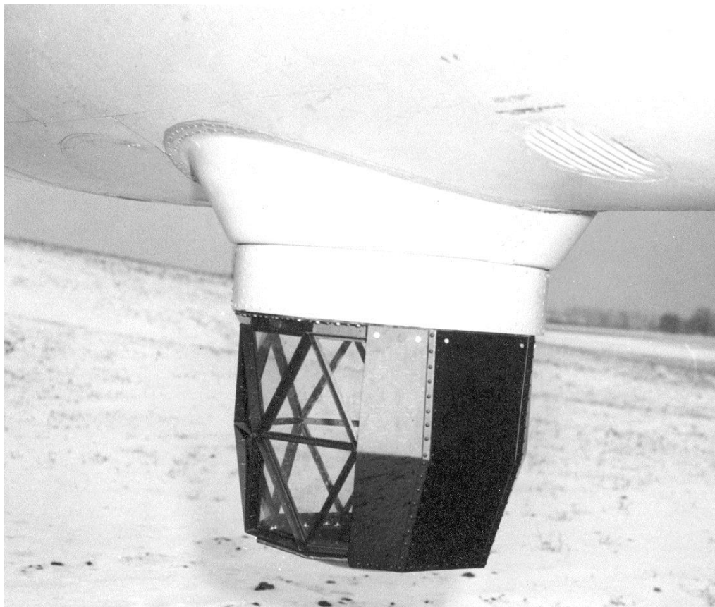
Bottom Clear IR Communications Radome
