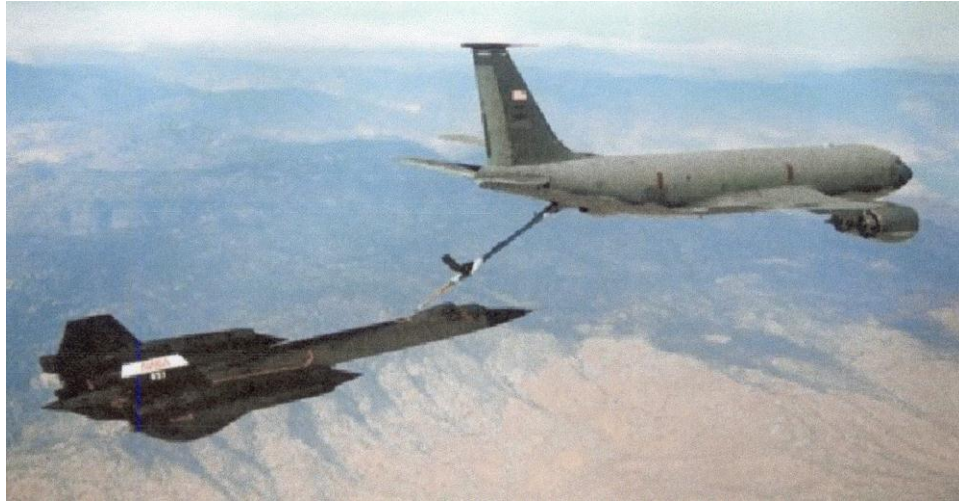
Figure 3 SR-71 Connecting Up with KC-135Q Tanker Equipped with AN/ARC-50 Radios
