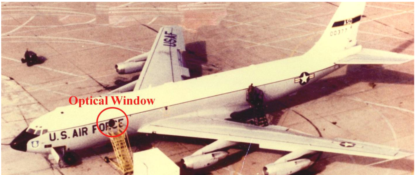
Figure 5a 4950 th Test Aircraft C-135-372 With Optical Window
