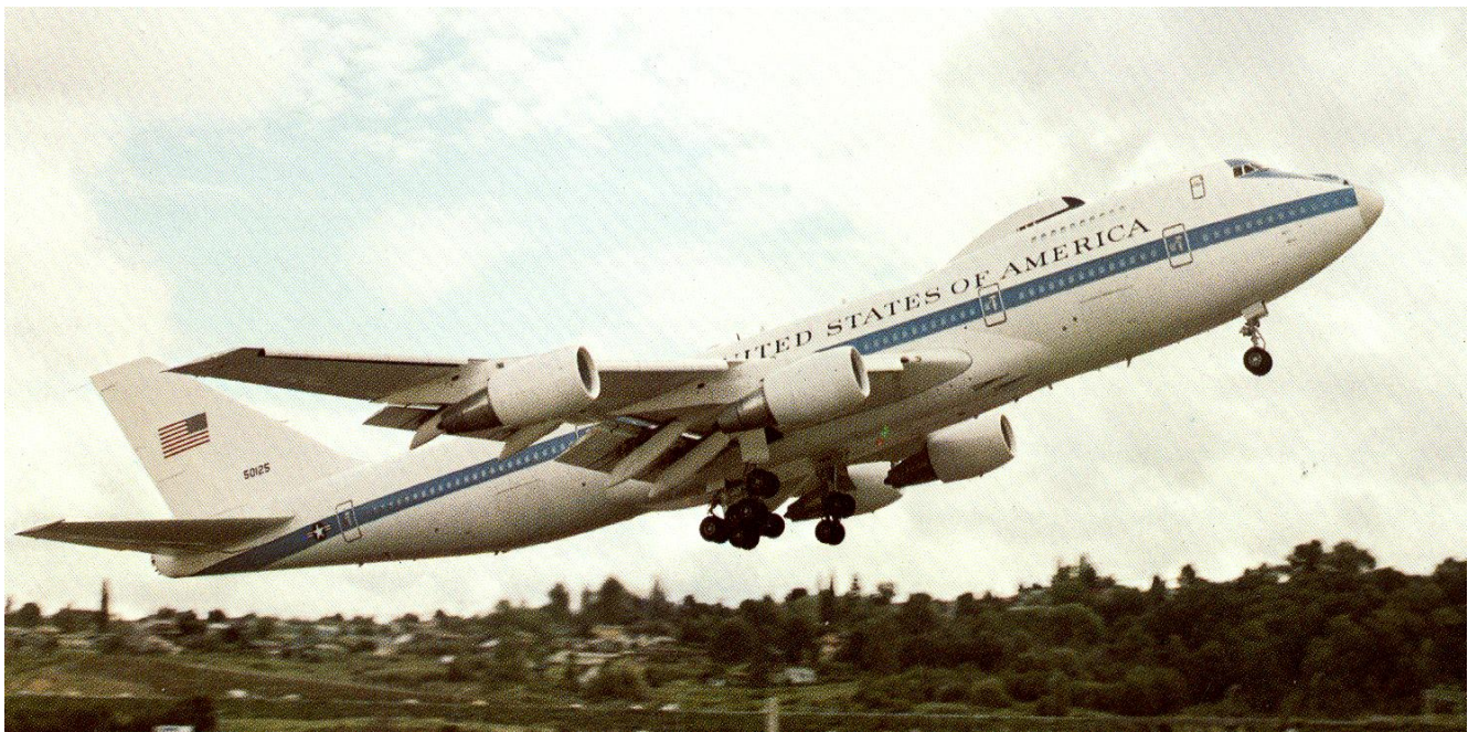
The Radome Forward of the Wing on the E-4B Houses the AN/ASC-24 SHF Antenna
