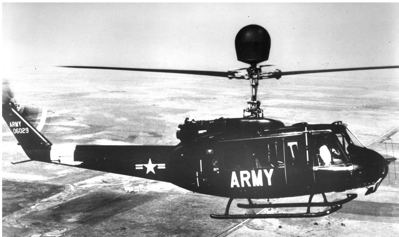
US Army Helicopter with SHF Satellite Communications Terminal
