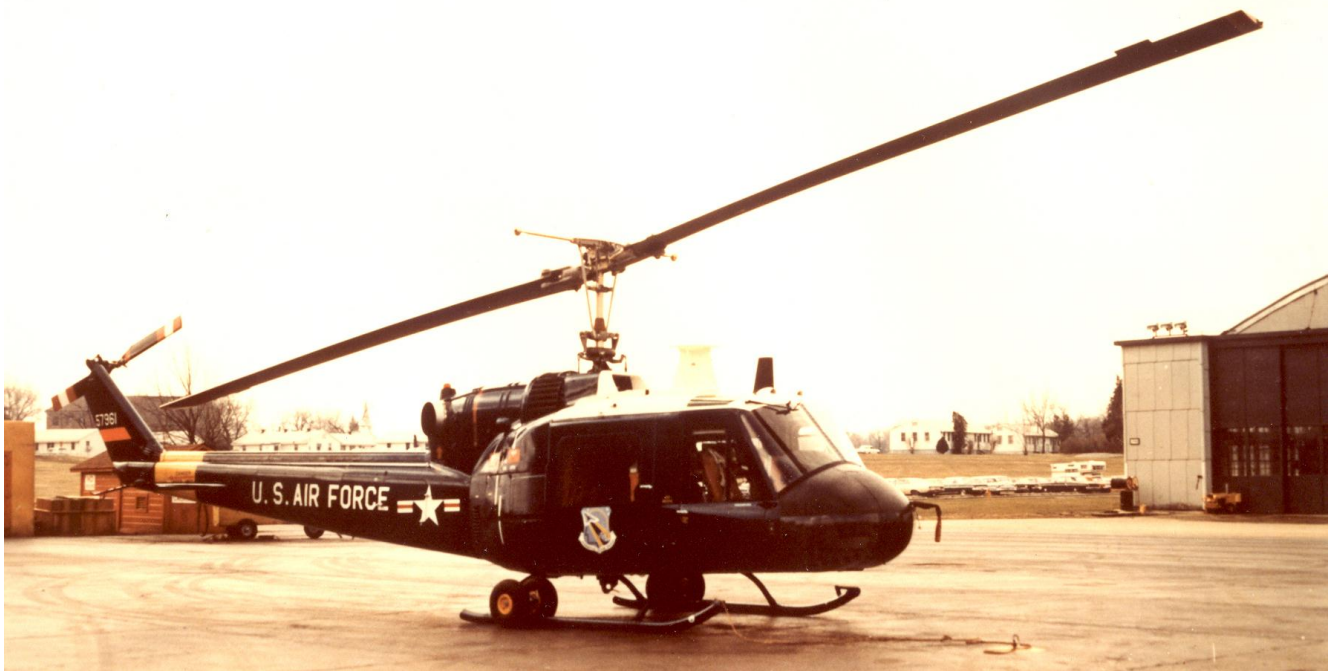
HU-1F Helicopter with Dorne Margolin VHF antenna atop cabin
