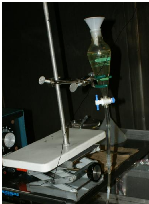
Figure 9. Separatory Funnel used to Control the Fuel Level
