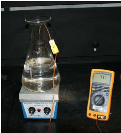
Figure 3. Fuel Sample being Mixed and Heated in Preparation for a Test
