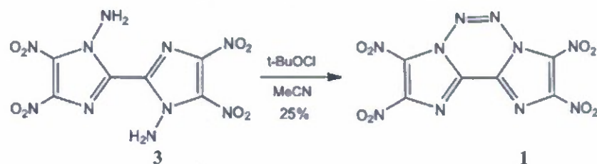
Scheme 2. Oxidative diamino coupling reaction of 3.
