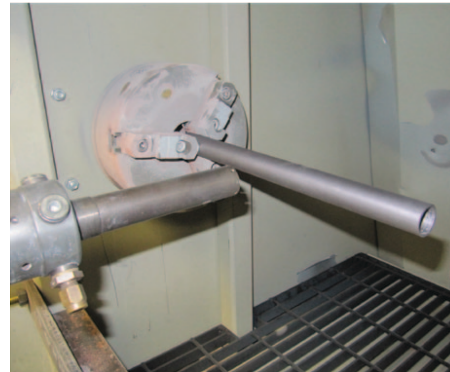
Cold spray consolidation of a tantalum tube.
