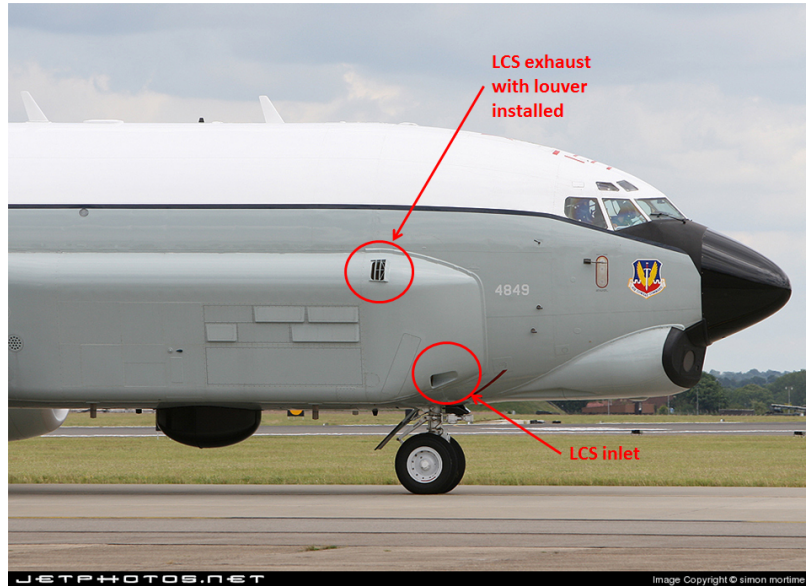
Figure 1.4: RC-135U Combat Sent showing LCS with louver installed over exhaust [1]
