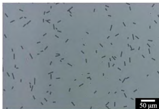
Fig. 4. Optical micrograph of glass rods dispersed in water in an anti-parallel rubbed cell.
