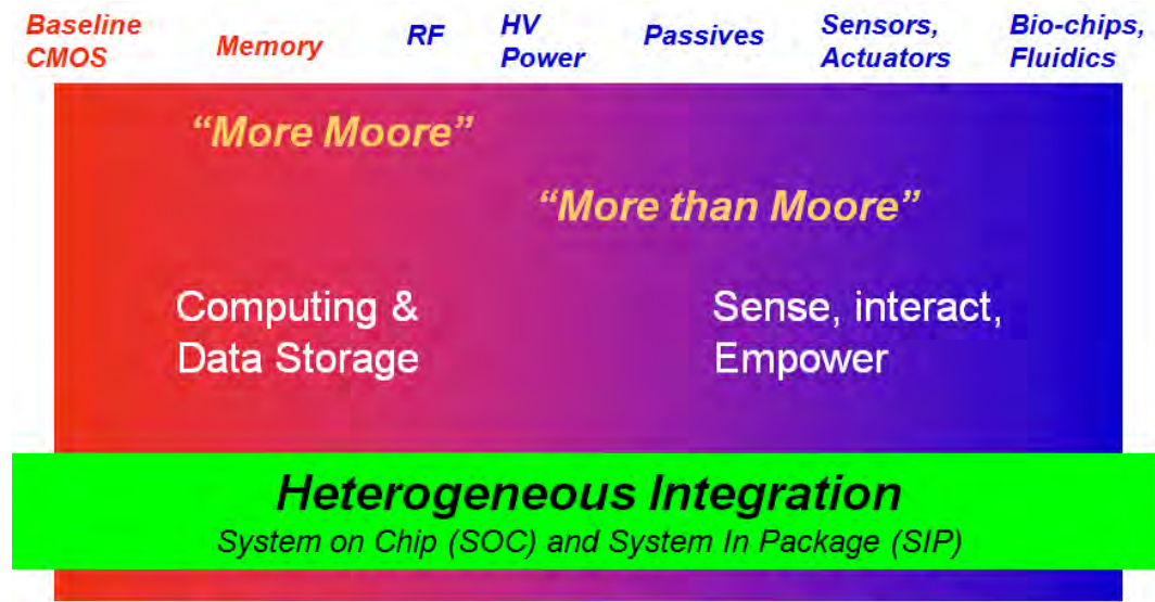
Figure F-1. “More-than-Moore” heterogeneous integration of functionality on the chip.
