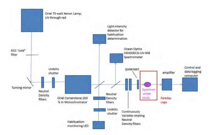
Figure 1. Electroretinography set up. The latest development is the construction of the CVNDF spectral intensity controller, which is currently being calibrated.
