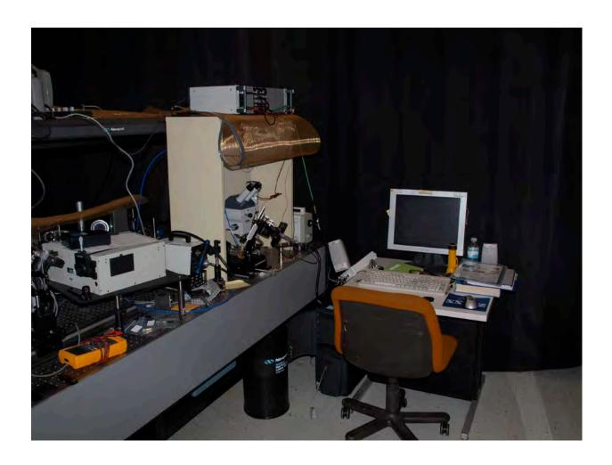
Figure 2: Photograph of the ERG set up. Monochromator on the left, work station with dissecting microscope in the old Faraday cage in center of photograph. NPI amplifier atop the Faraday cage. The addition of a linear polarizer will permit investigation of polarization sensitivity.
