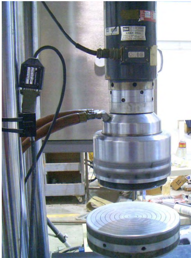
Figure 34. 50 kip loading machine.
