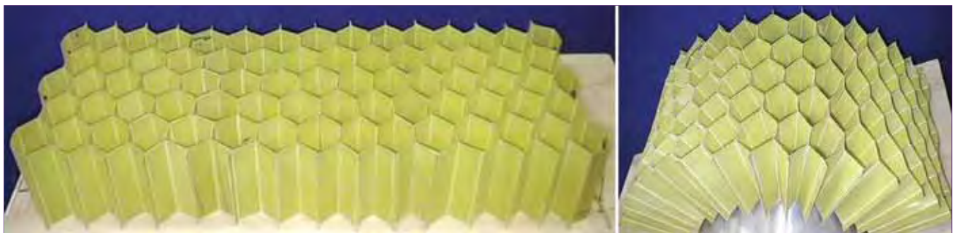
Figure 1 Photographs Showing Linear and Radial Deployment of the DEA
