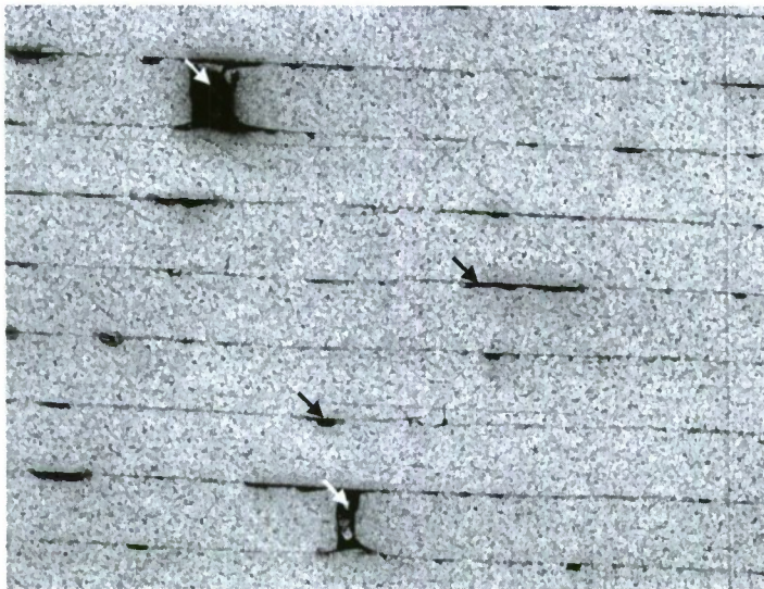
Fig.12. Microstructure of an Al 3003 UC sample made using the default foil width setting of 0.9411 inch. White arrows show defects at foil junctions. Black arrows show unbonded regions along layer interfaces.
