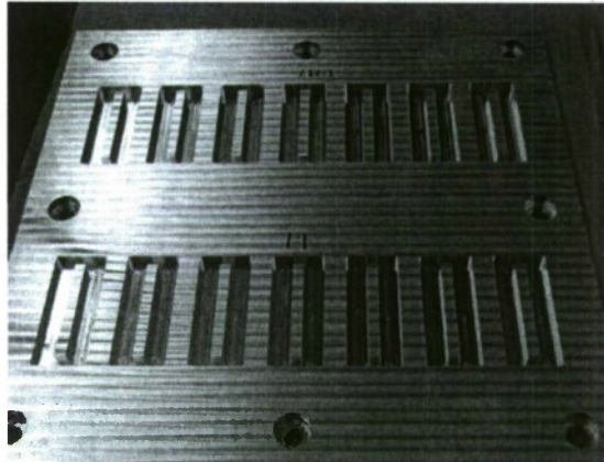
Fig. 16. Aluminum rib in channel plate before being filled with support materials.
