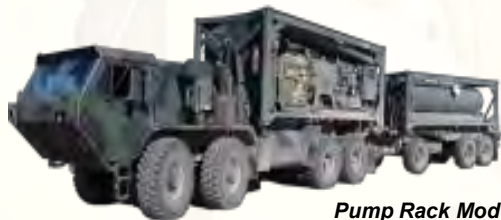
Pump Rack Module (PRM) and Tankrack Module (TRM)
