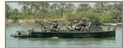
Bridge Erection Boat (L)
