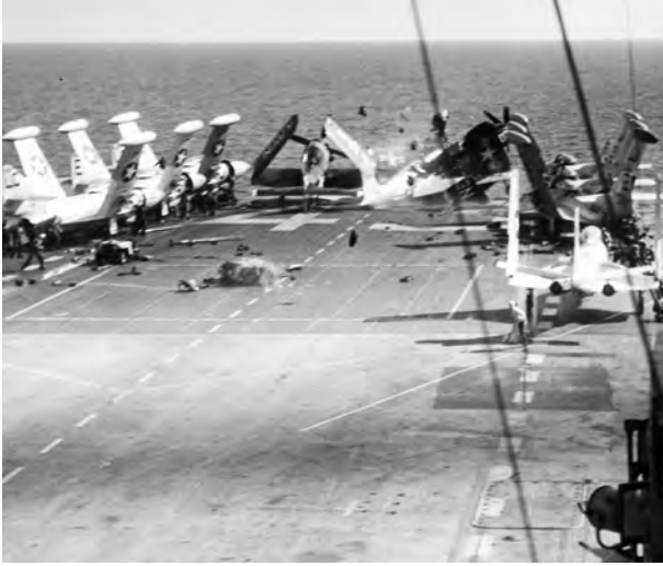
The F2H-1 has collided with the two Skyraiders; it will push both overboard and then go overboard itself. The driver of the jeep tractor on the centerline is miraculously alive.
