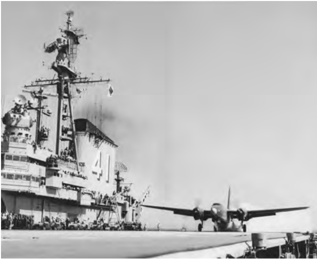
A modified Lockheed P2V Neptune patrol bomber takes off from the USS Midway (CV 41) in April 1949, accelerated to launch speed by JATO units.
