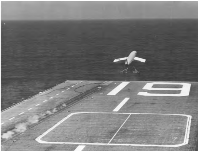
A Regulus-1 air-breathing, long-range missile catapulted from Hancock in 1957. The trolley holding the missile and pulled by the steam catapult is lost when the missile is launched.
