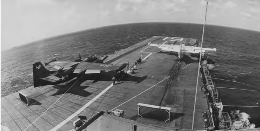
Two AJ-1 Savages on Hancock in late November 1955. The plane on the starboard catapult is being launched; that on the port catapult is waiting its turn. Note the early-model jet-blast deflectors.
