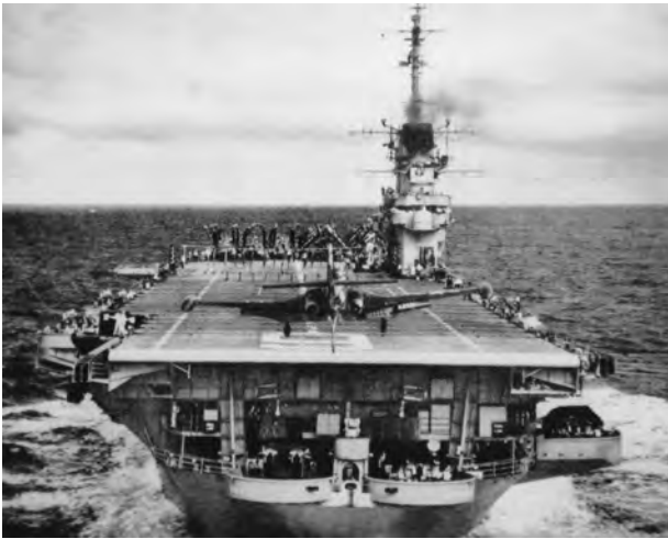
A Grumman F9F Panther jet lands on Essex (CV 9). The athwartship barrier is up, but from the pilot's view he's landing into a deck full of aircraft.
