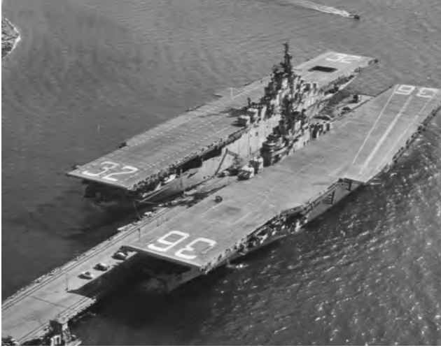
An unmodified carrier, USS Leyte (CV 32), on the left and a carrier given an angled deck, USS Antietam (CV 36), on the right, October 1954. As Vice Adm. Robert Dunn noted to the authors, the angled deck eliminated the demand from pilots for a flush-deck carrier.
