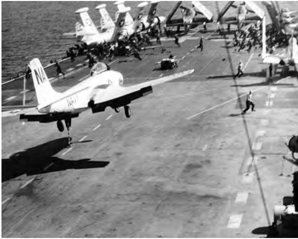
What every pilot feared—missing the arresting gear and vaulting over the barrier. The F2H-1 is headed for two Skyraiders parked at the forward end of the flight deck of USS Coral Sea (CV 43). The flight deck crew members are running for their lives.
