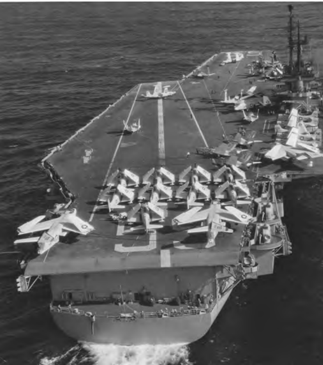
USS Forrestal (CVA 59), the first of the new postwar U.S. Navy carriers, with an angled deck, steam catapults, deck-edge elevators, and a mirror landing aid. Note the large Douglas A3D Skywarriors.
