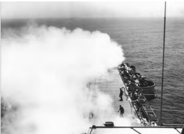
The first test of a U.S. Navy steam catapult at sea, July 1954. USS Hancock (CVA 19) is launching . . . what? The plane is completely obscured by steam leaking from the catapult.
