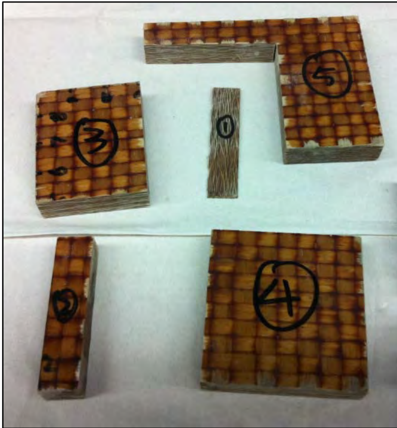
Figure 3.17. Various Different Cuts HJ1 Coupons
