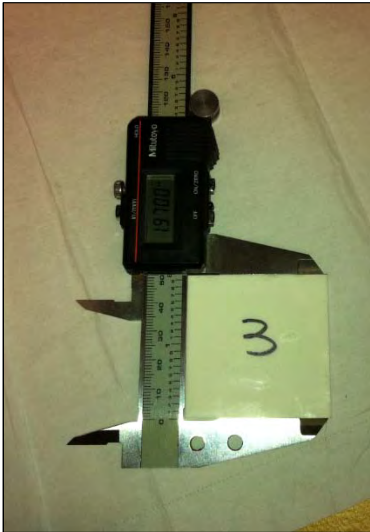
Figure 3.16. Measuring the Dimensions of Ceramic Coupon #3
