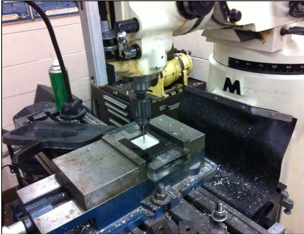
Figure 3.30. Ceramic Coupon Being Drilled
