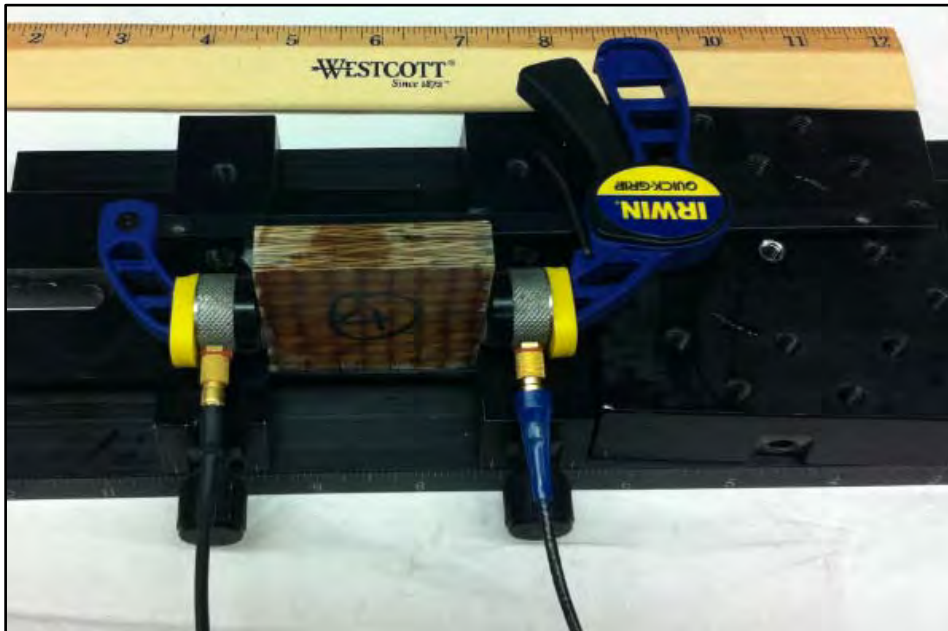
Figure 3.19 Another top View of the Composite Coupon on the Mounting Platform with PZT Sensors Clamped on to the Coupon
