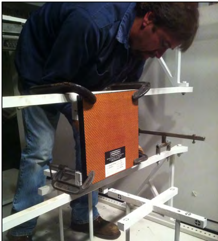
Figure 3.46. 46 th Test Group Personnel Clamping on the Armor System
