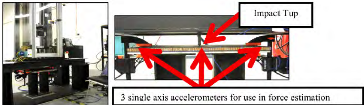
Figure 2.14. Passive Structural Health Monitoring on S-2 Composite Armor
