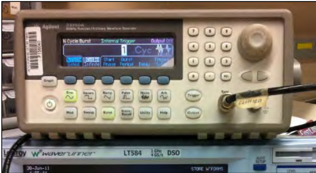
Figure 3.20. Waveform Generator Used to Create Input Wave Propagations
