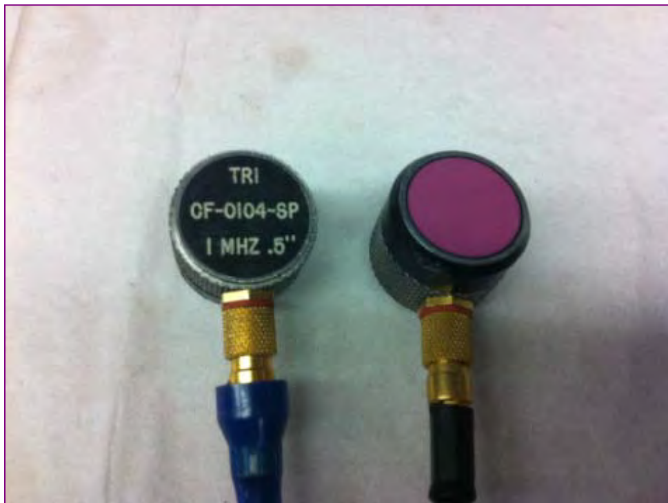
Figure 2.5. PZT Sensor used to Induce and Collect Wave Propagation
