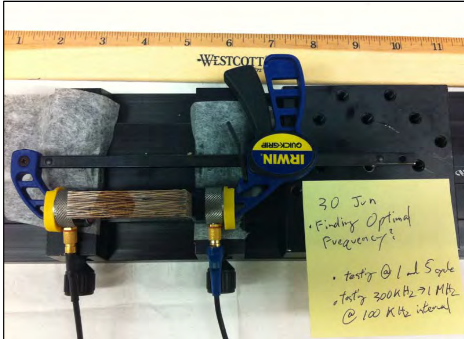
Figure 3.18. Top View of the Composite Coupon on the Mounting Platform with PZT Sensors Clamped on to the Coupon
