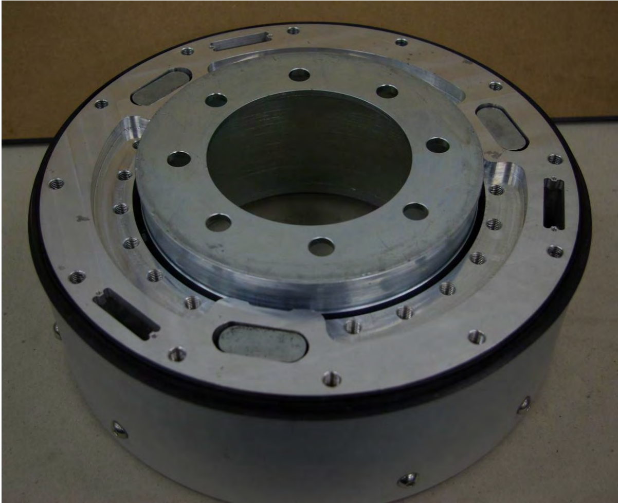
Figure 8 - Assembled wheel force transducer inside view (vehicle side)
