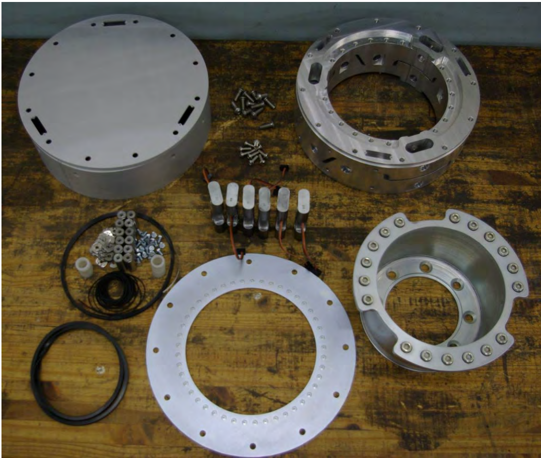
Figure 6 - Components of a wheel force transducer
