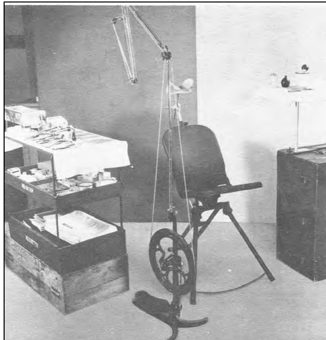
Figure 1. The equipment set depicted is very similar to dental sets seen in photos from the time of the Spanish American War until the beginning of Vietnam War. Commonly referred to as a "Chest 60" Field Dental Set, the instruments and equipment were carried in boxes and could be used without electricity, e.g., using natural light and foot treadle powered dental handpiece. As electricity became more accessible a motor was added to the belt driven handpiece and patient lights were added. Reproduced from United States Army Dental Service in World War II . 2
