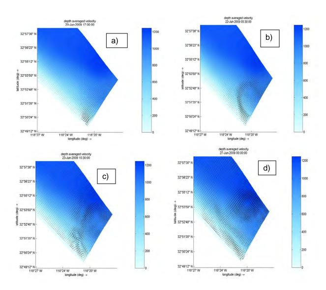
Figure 1: Evolution of a boundary instability: vectors of depth averaged currents. Time progresses from a) to d), at which point the simulation becomes completely unstable.
