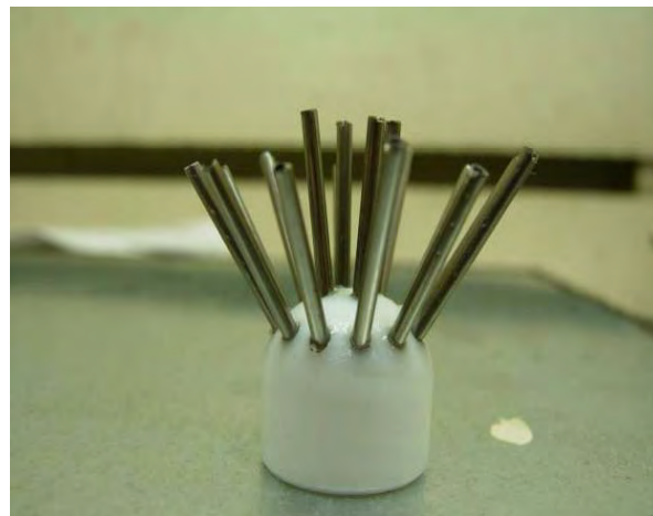
Figure 3-6. Effluent manifold, made of Teflon, used to connect the effluent lines. Stainless steel needles were used to connect this manifold to the Teflon-lines effluent lines.
