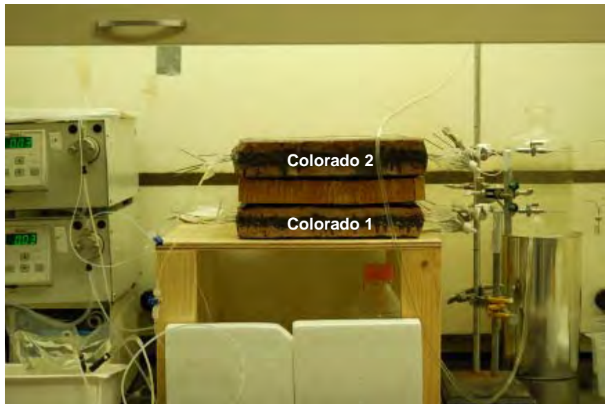
Figure 3-9. Experimental fracture apparatus constructed from sandstone blocks (influent manifold on the left, and effluent manifold on the right). Each rock was approximately 29 cm long (L) x 29 cm wide (W).
