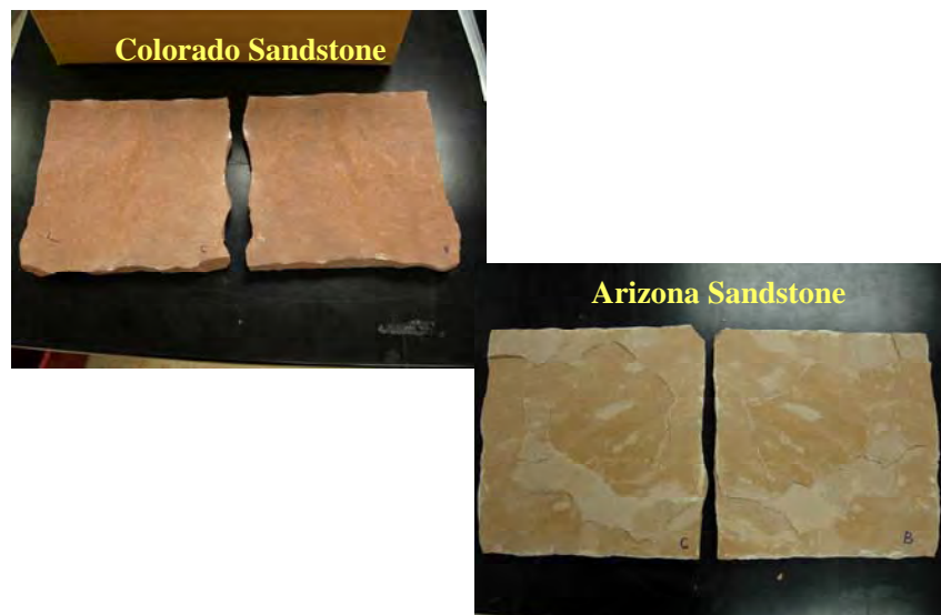
Figure 3-4. Fracture roughness. Internal view of fractures for the Arizona and Colorado sandstones.
