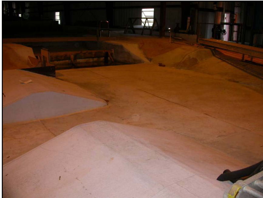
Figure 2.31. Test basin for 1 : 16 scale physical model tests.
