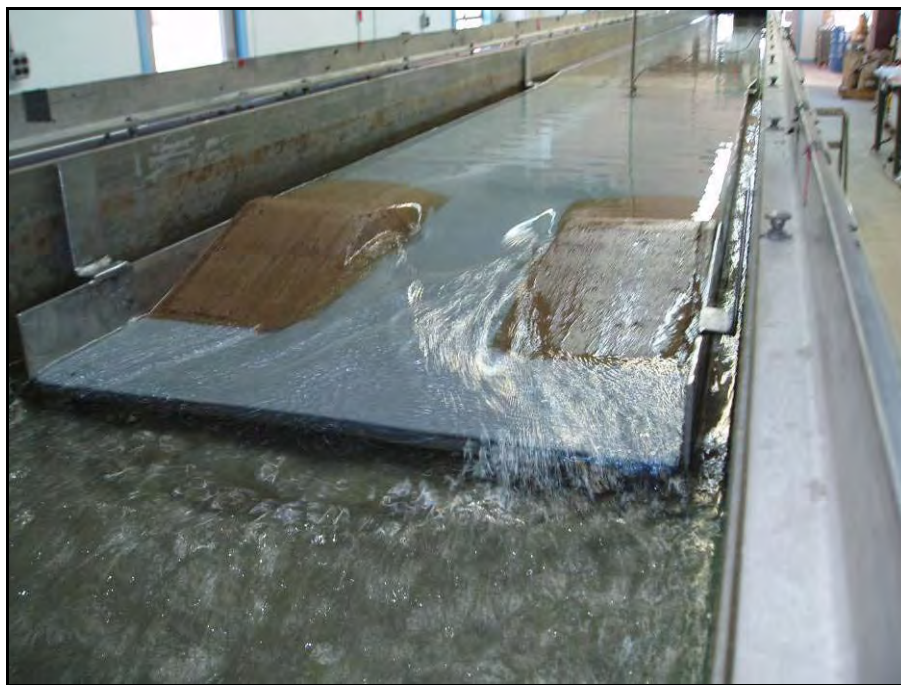
Figure 2.25. Photo of flow through small-scale (1 : 50) breach.
