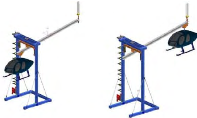
Figure 6-9: Illustration of full-scale crash test approach. Reprinted from Reference [90].
