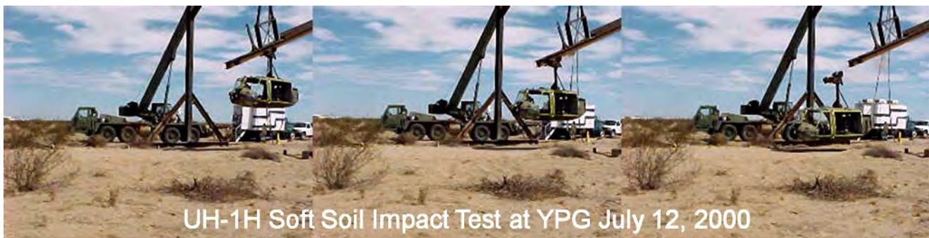
Figure 6-8: Full-scale crash tests at YPG for impact test of a Huey onto water and soil
