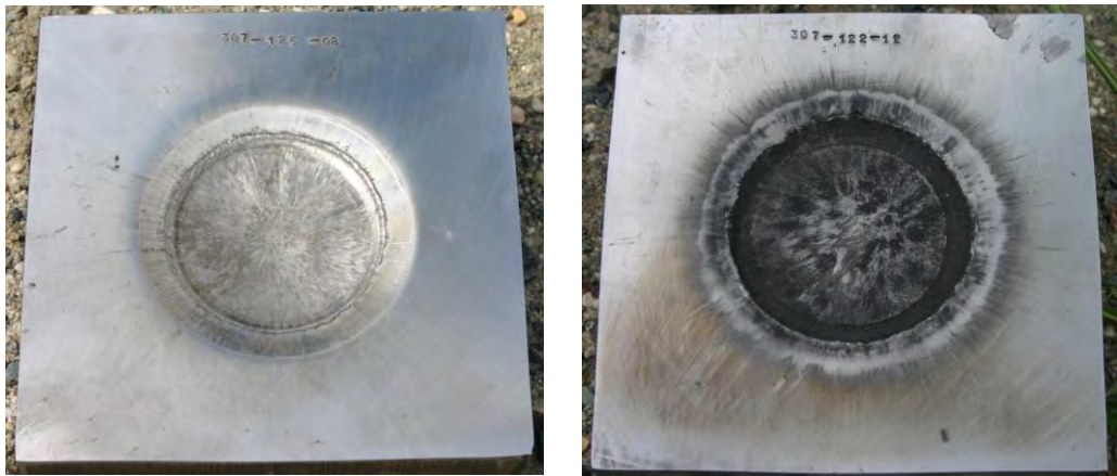
Figure 18. Witness block dents of 8.23-mm (left) and 10.99-mm (right) in IMADGTs with 70.08- and 68.40-mm gaps, respectively, for PBXN-109 containing Dyno Nobel RS-RDX
