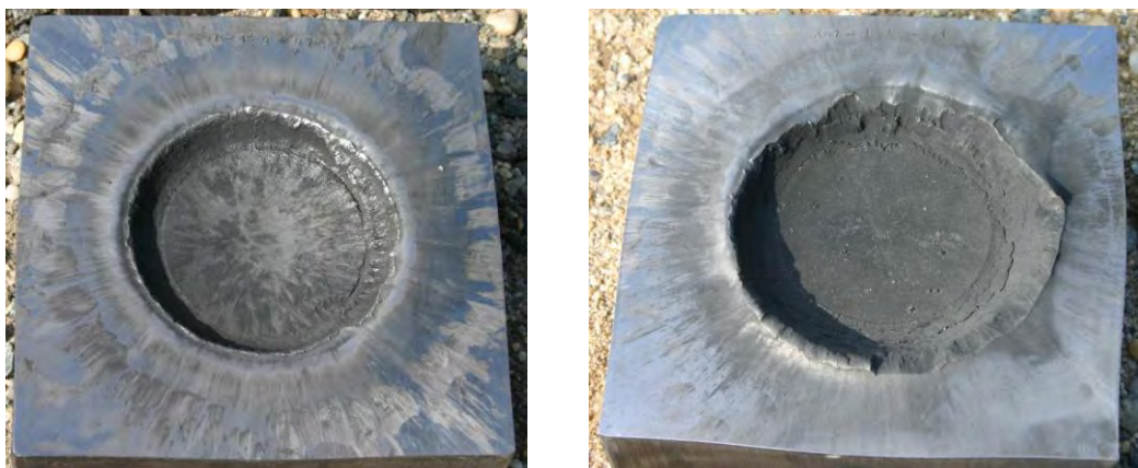
Figure 19. Witness block dents of 13.74-mm (left) and 16.90-mm (right) in IMADGTs with 64.06- and 2.54-mm gaps, respectively, for PBXN-109 containing Dyno Nobel RS-RDX
