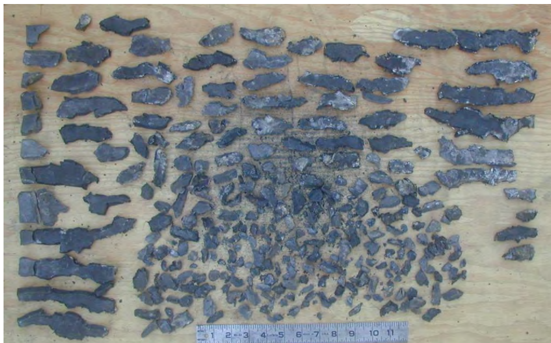
Figure 14. ELSGT acceptor tube fragments (gap end shown to the left) for PBXN-109 filled with Dyno Nobel RS-RDX and subjected to a donor shock attenuated by an 81.27-mm gap
