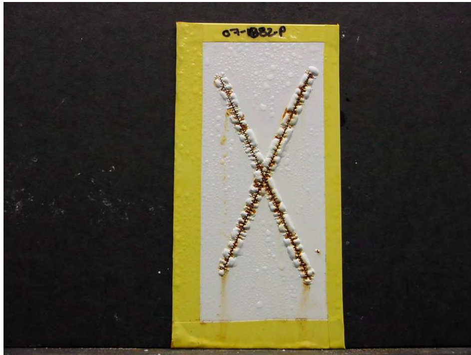
Figure 25. LTCPC Cyclic Corrosion Resistance Test Outcome – Steel
