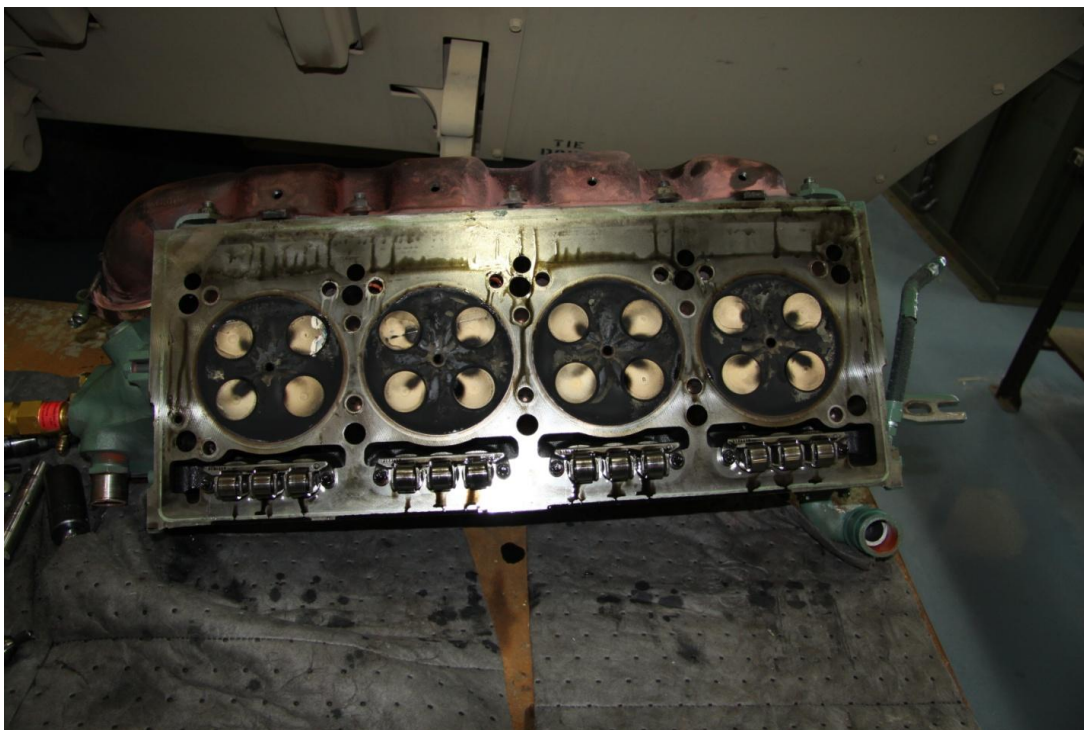
Figure 14. JP-8/FT engine cylinder heads 1,3,5,7 with debris build-up
