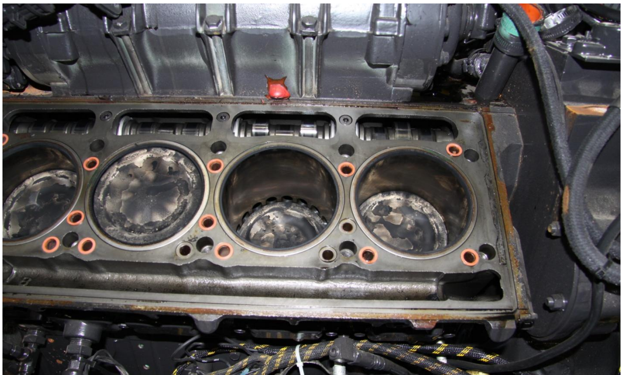
Figure 17. JP-8 piston cylinders with excess build-up on piston heads for cylinders 2,4,6,8
