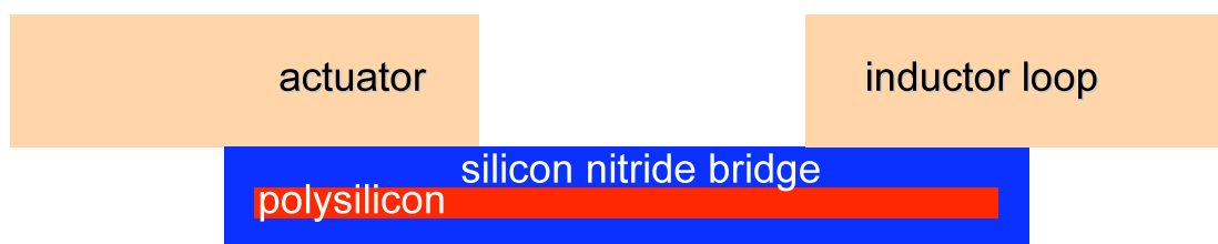
Figure 37: Diagram of electrically isolated, mechanically coupled bridge, side view
