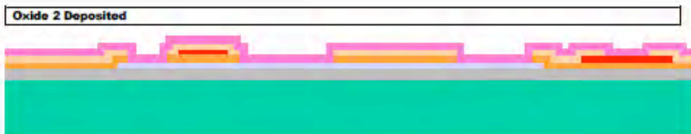
FIGURE 1.8. A second sacrificial layer (Oxide 2), 1.1µm of PSG, is deposited and annealed at 1050°C for 1 hour.
