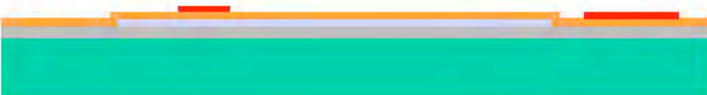
FIGURE 1.5. The wafers are coated with photoresist and the second level (POLY) is lithographically patterned. Reactive ion etching (RIE) is used to remove the unwanted polysilicon. After the etch is completed, the photoresist is removed.
