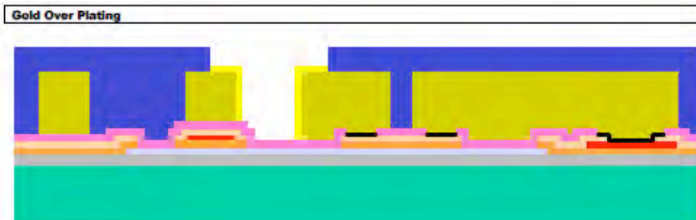
FIGURE 1.14. A 1-3µm gold layer (Sidewall Metal) is electroplated using the GOLDOVP photoresist mask as a stencil.
