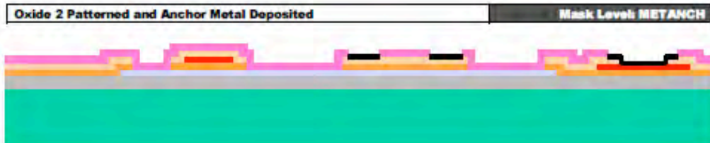
FIGURE 1.9. The wafer is coated with photoresist and the fourth mask level (METANCH) is lithographically patterned. The Oxide 2 is wet etched and a thin metal layer (Anchor Metal) consisting of 10nm Cr + 25nm Pt is deposited. A liftoff process is used to remove the photoresist and leave Anchor Metal only in the bottom of the Oxide 2 openings formed from the METANCH mask level.
