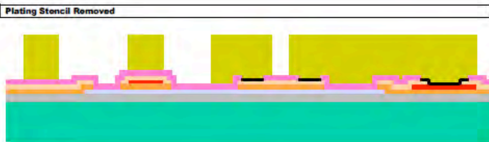
FIGURE 1.12. The photorecist stencil is then chemically removed.
