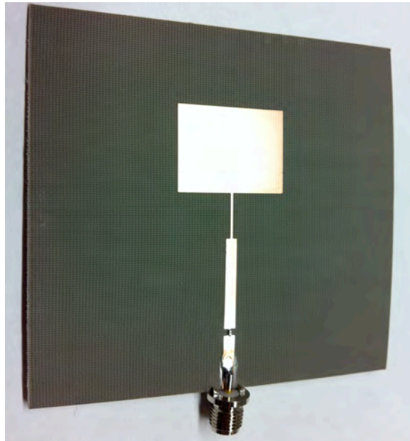
Figure 20: 5.5 GHz patch antenna with discrete reactive load
