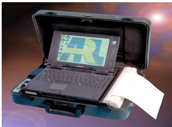
Figure 1. A photograph of the portable FALCon system, with a laptop, a scanner, and a battery pack.
