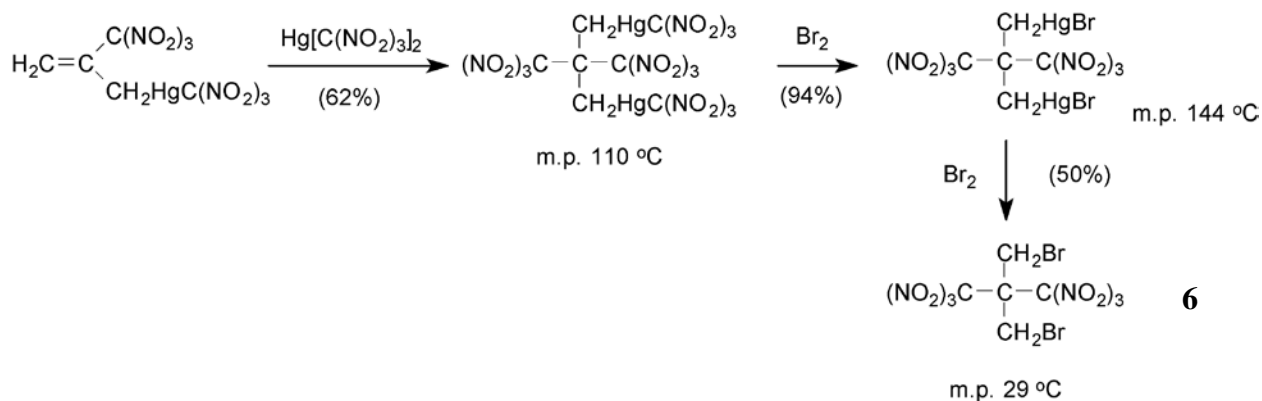
Scheme 7. Preparation of a 1,1,1,3,3,3-hexanitropropane derivative ( 6 ) [39]
