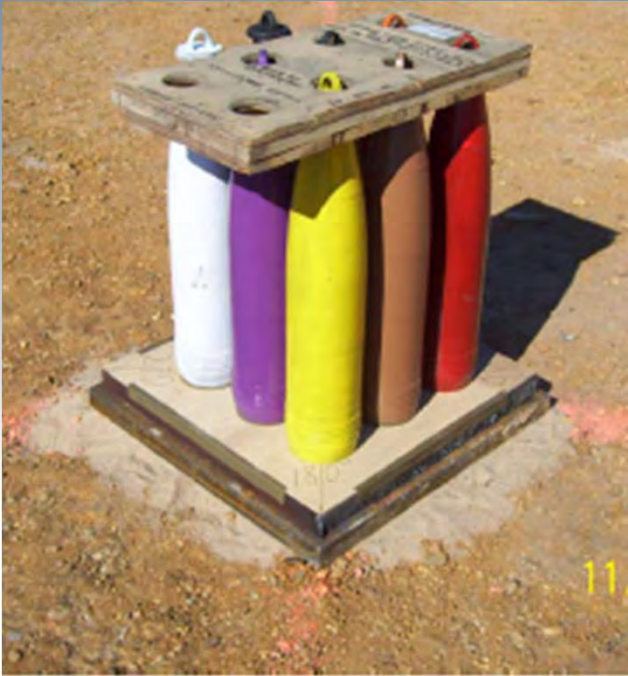
Test Setup Un-Confined Sympathetic Detonation Test
