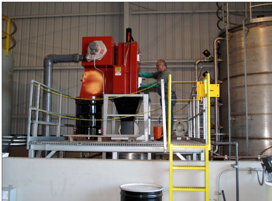
Figure 5-11. View of platform and ladder with installed can crusher.
