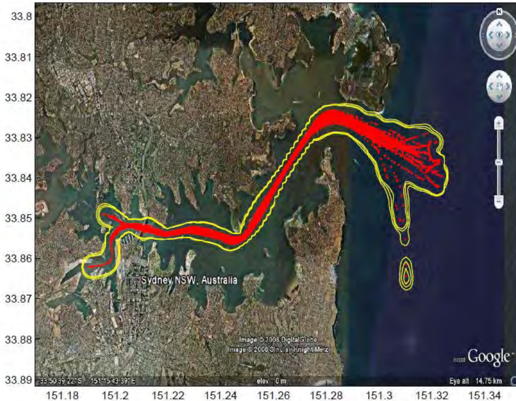
Figure 4 - Two-dimensional motion patterns of maritime traffic entering Port Jackson with anomaly decision boundaries [Ristic et al., 2008]
