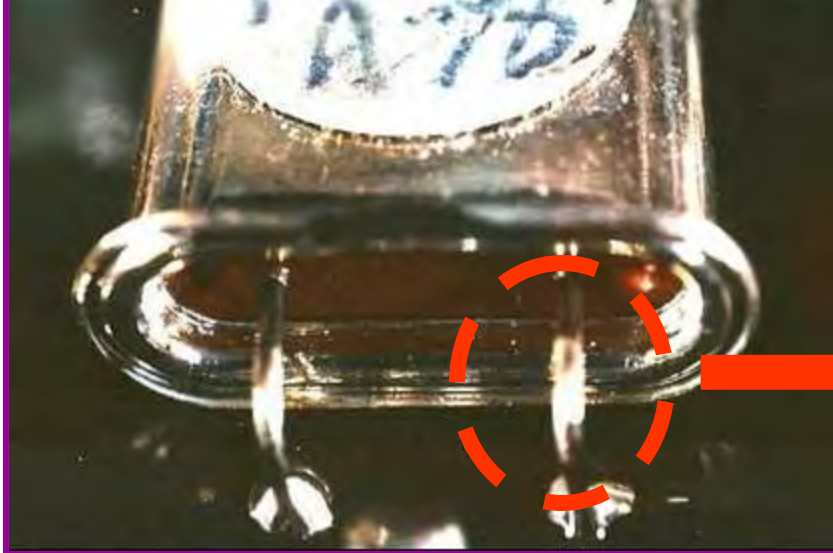
Crystal with Tin-Plated Kovar Leads (with Nickel Underplate)
