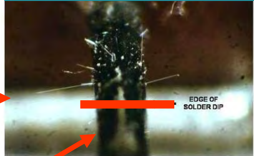
Tin Whiskers (~60 mils) Grew on NON-Dipped Region Shorting to Case Causing Crystal to Malfunction
