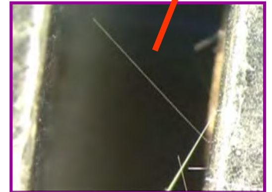
Tin Whiskers Growing on Armature Of Relay Produced Metal Vapor Arc Resulting in Destruction of Device
